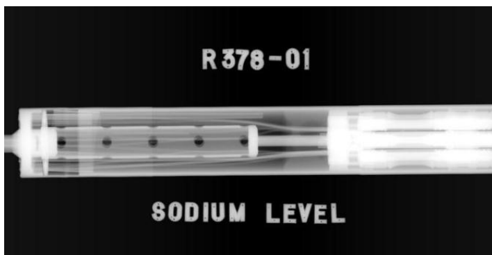
Figure 17: X-ray of CORONIS capsule to check for correct sodium level
