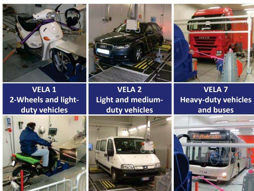
**Figure 2.1: VELA facilities** - The Vehicle Emission Laboratories, JRC - Italy
