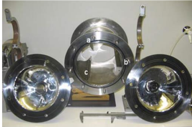
Figure 71. Photograph showing the high-gloss polished inside of the dustiness drum. Also note the three lifter vanes marked a. b. and c at each 120° in the drum.
