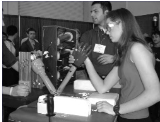
Figure 2: An EAP driven arm made by students from Virginia Tech and the human opponent, 17-year old student.
