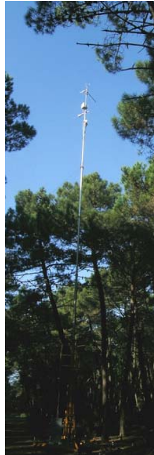
Fig.47: Trailer mast in San Rossore that holds the sonic anemometer and Infra Red Gas Analyser (IRGA) used for flux measurements (on the left picture in retracted configuration for service, on the right at measurement position).
