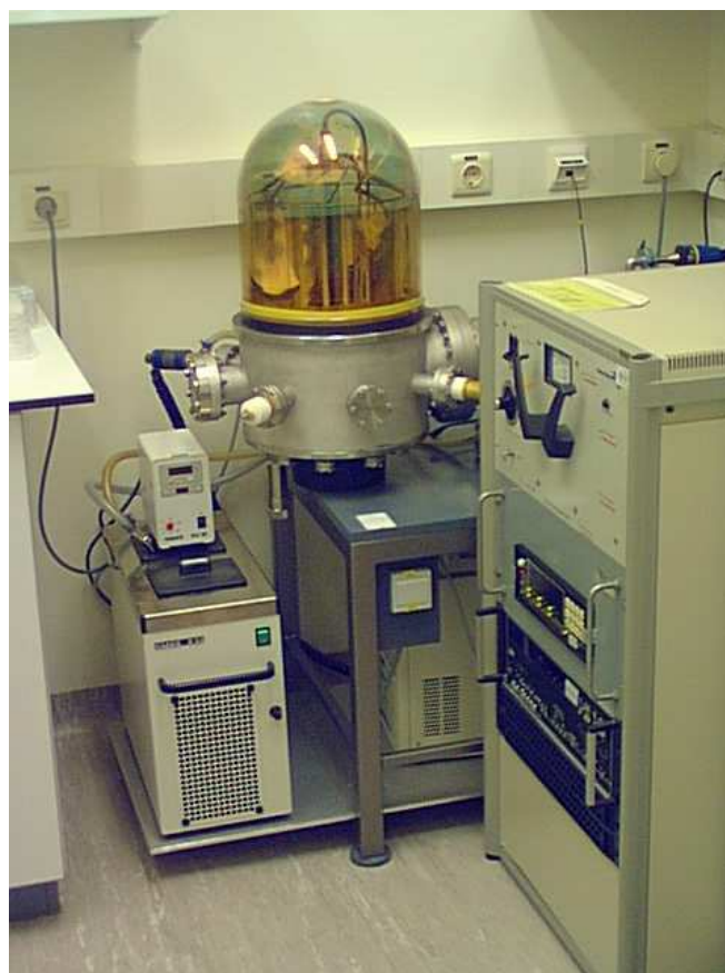
Figure 4: Vacuum evaporator in an IRMM lab where Mr A. Dirican (LTT) was being trained on Standardisation of activity and decay data measurements.
