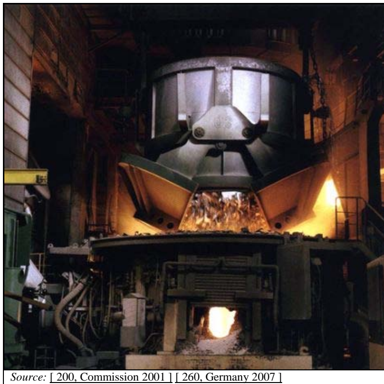
Figure 8.2: Electric arc furnace charging
