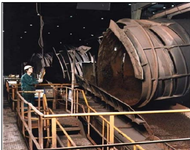
Figure 4.1: Balling drum as part of a pelletisation plant where the green pellets are formed
