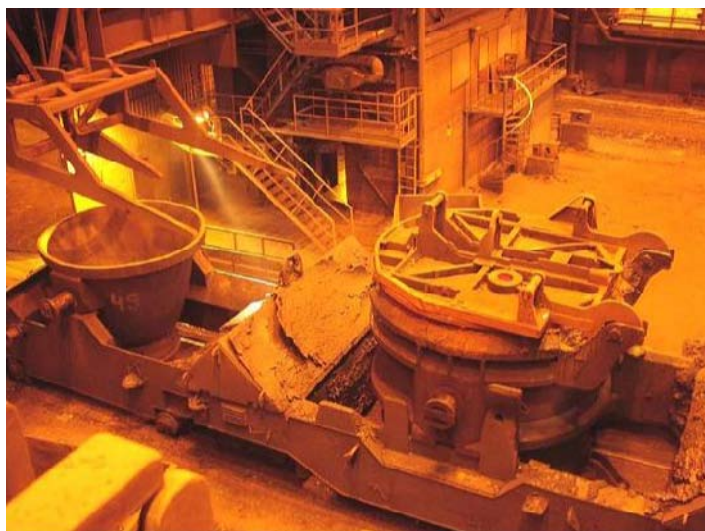
Figure 7.24: Automatic ladle lid system
