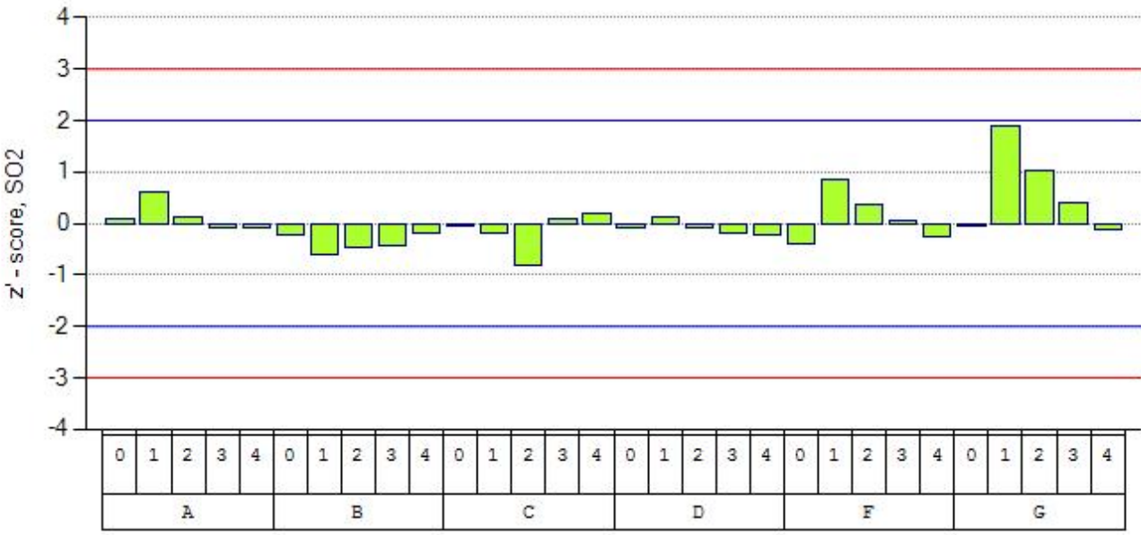
Figure 3: The z'-score evaluations of SO 2 measurements Scores are given for each participant and each tested concentration level (run). Run number order (with nominal concentration) is: 0 (0 nmol/mol), 1 (120-140 nmol/mol), 2 (40-50 nmol/mol), 3 (15-25 nmol/mol), 4 (4-7 nmol/mol). The assessment criteria are presented as z'=\pm 2 (blue line) and z'=\pm 3 (red line). They represent the limits for the questionable and unsatisfactory results.
