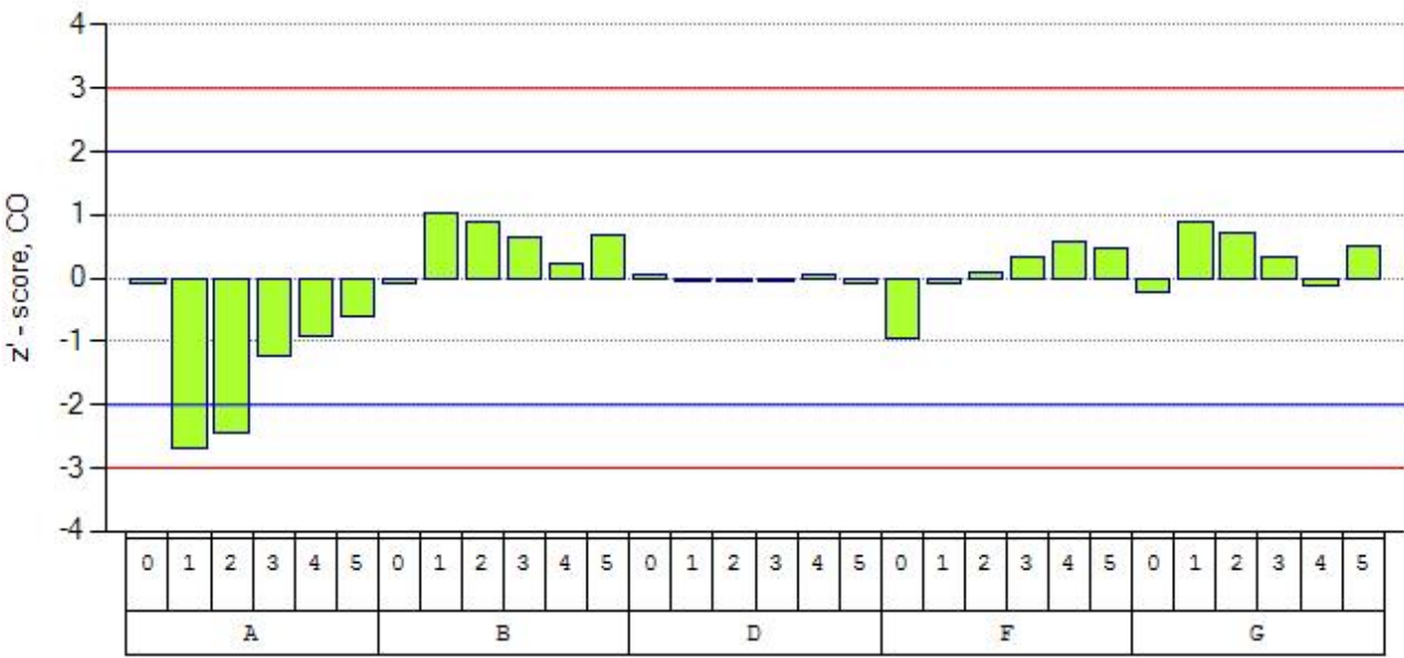
Figure 4: The z'-score evaluations of CO measurements Scores are given for each participant and each tested concentration level (run). Run number order (with nominal concentration) is: 0 (0 μmol/mol), 1 (6-9 μmol/mol), 2 (5-8 μmol/mol), 3 (2-4 μmol/mol), 4 (0.5-2 μmol/mol), 5 (4-5 μmol/mol). The assessment criteria are presented as z'=\pm 2 (blue line) and z'=\pm 3 (red line). They represent the limits for the questionable and unsatisfactory results.
