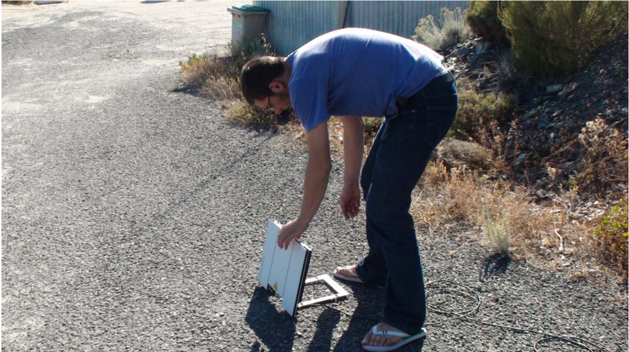
Figure 33 – Satellite Communications Terminal Thrane & Thrane Explorer E700 being deployed.
