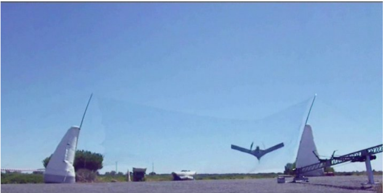
Figure 26 – UAV after landing. After crashing against the net the UAV remains suspended until the operations team collects the UAV.
