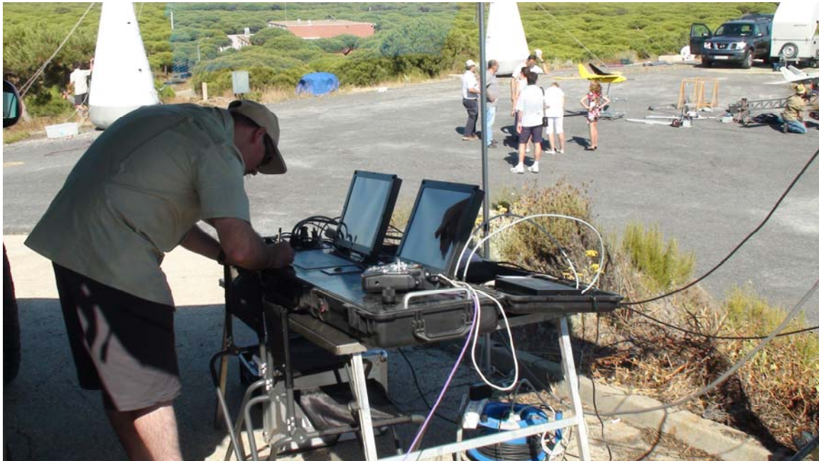
Figure 28 - UAV Control unit with 2 displays and 1 joystick.
