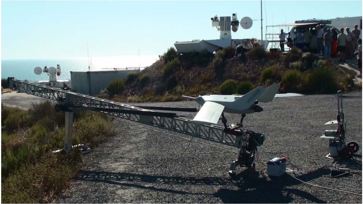
Figure 22 – UAV Launch Pad from a different perspective. On the top left and right hand sides of the picture two target trackers can be seen. These trackers were used to track the UAV and the small boat deployed during the experiment.
