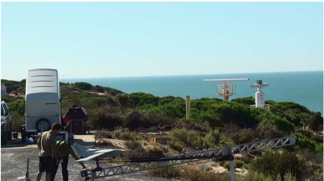
Figure 21 – Profile view of the UAV Launch Pad with the UAV ready for launch.
