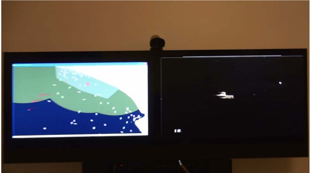
Figure 44 – On the left hand side, the display of AIS information. On the right hand side the real time video from the SIVE camera.
