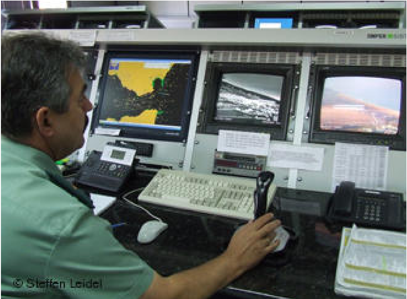
Figure 40 – Guardia Civil SIVE Station in Huelva-Spain. Control of the radar, AIS and SIVE cameras data.
