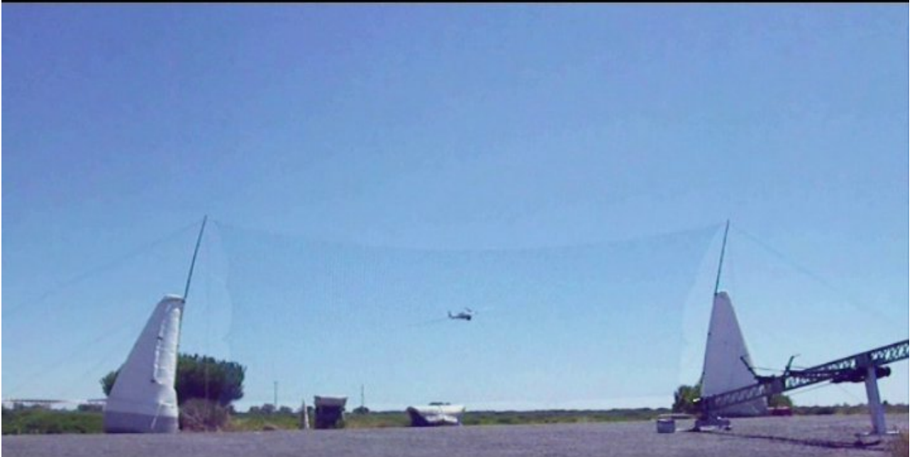
Figure 25 – UAV Landing System. The Landing System consists of a net kept vertical by two lateral inflatable pillars. In this picture the UAV is just about to land on the net.
