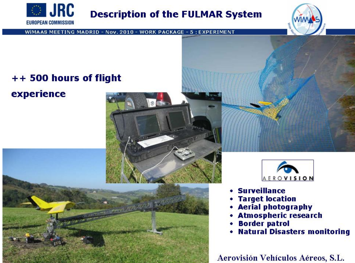
Figure 5 - UAV FULMAR System. On the bottom left the launch system. In the middle the command and control system. On the top right the net landing system.
