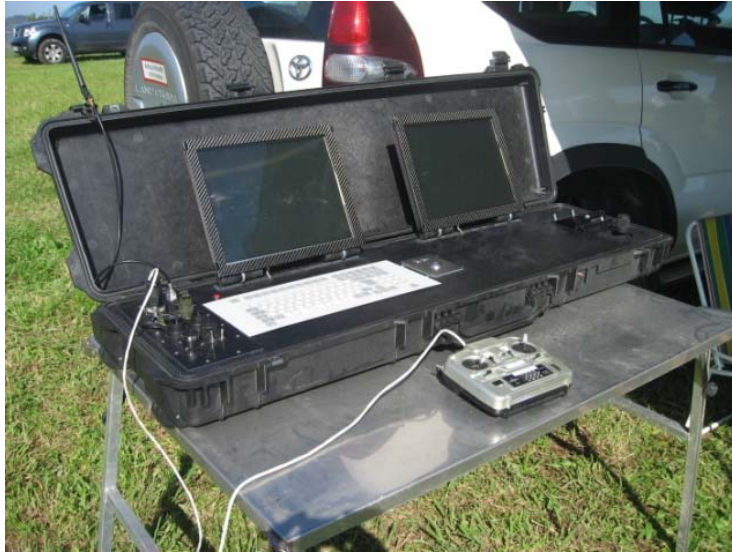
Figure 27 – UAV Control unit with 2 displays and 1 joystick.
