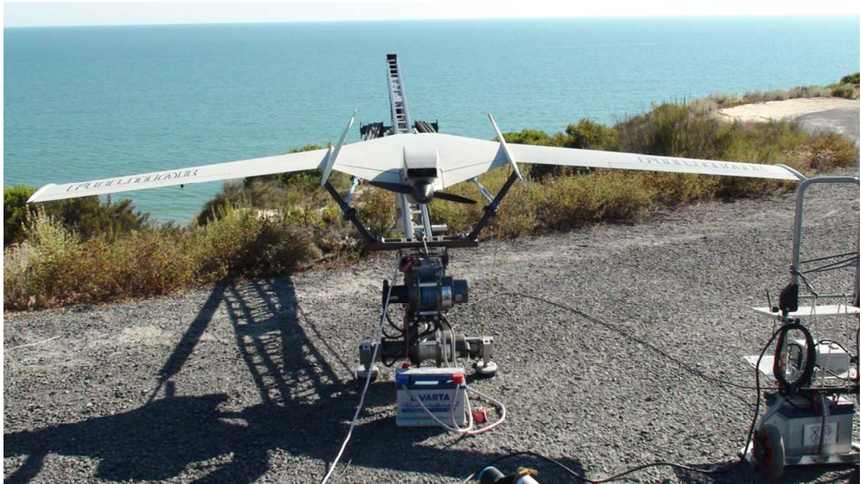
Figure 20 – UAV on launch pad ready for launch.
