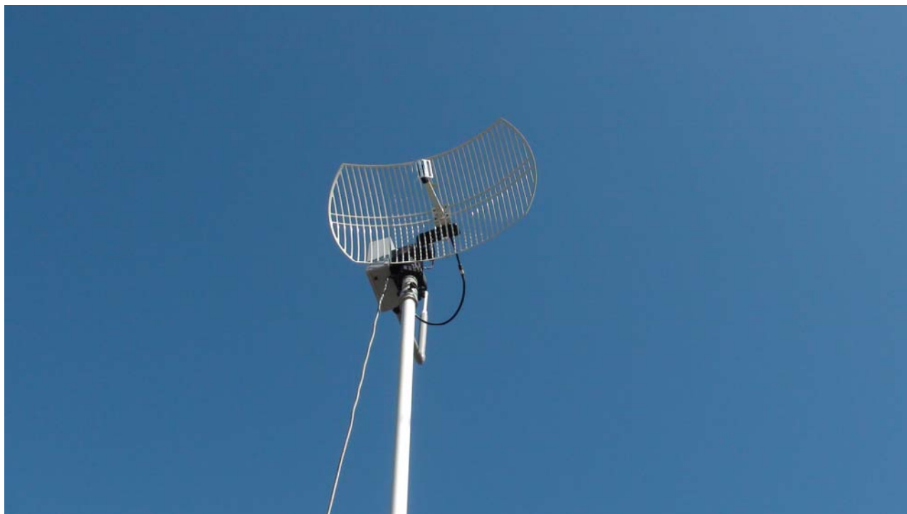
Figure 29 – Ground Control System Antenna.
