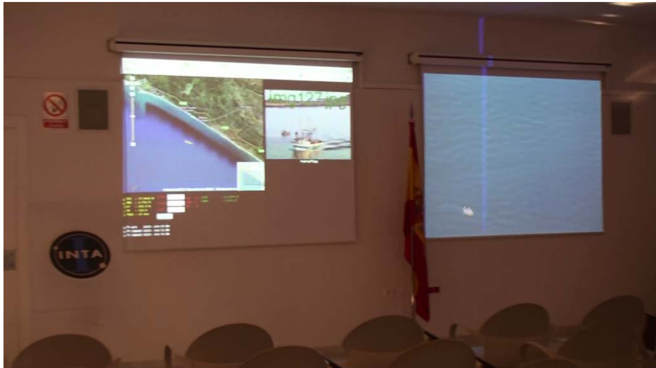
Figure 43 – On the left hand side, the display of the UAV position and the UAV video transmitted via Satcom. On the right hand side, the UAV video from the ground control system.
