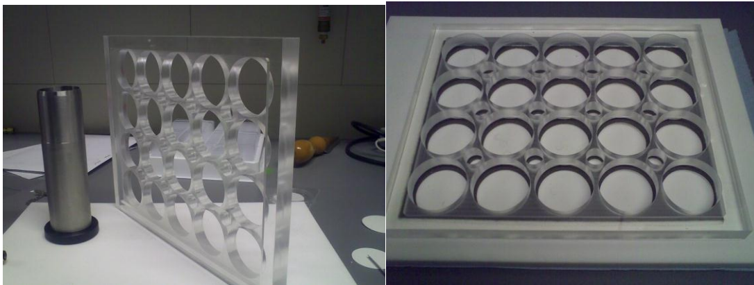
Figure 1.– Mould and tools for the subdivision of the high volume sampled filter
