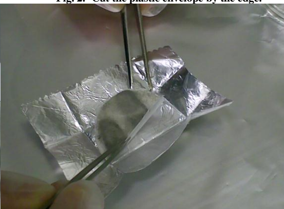
Fig. 4.- Unwrap the aluminium foil to get the filter
