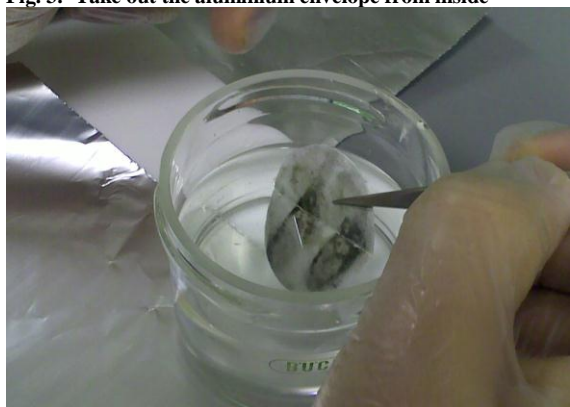
Fig. 5.- Unfold the filter and introduce it into your container for extraction
