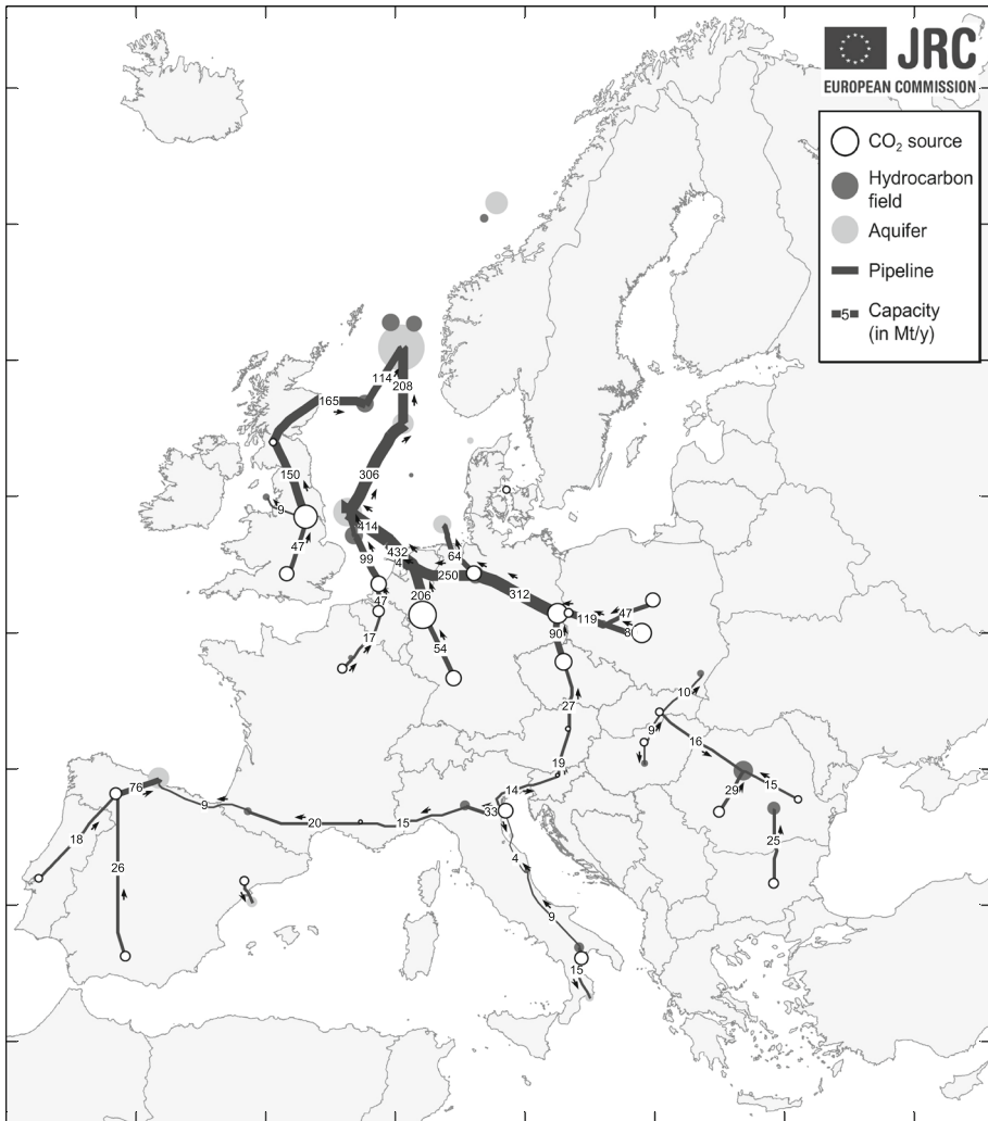
Fig. 3 CO 2 pipeline network in 2050, assuming joint international optimisation without participation of Denmark
