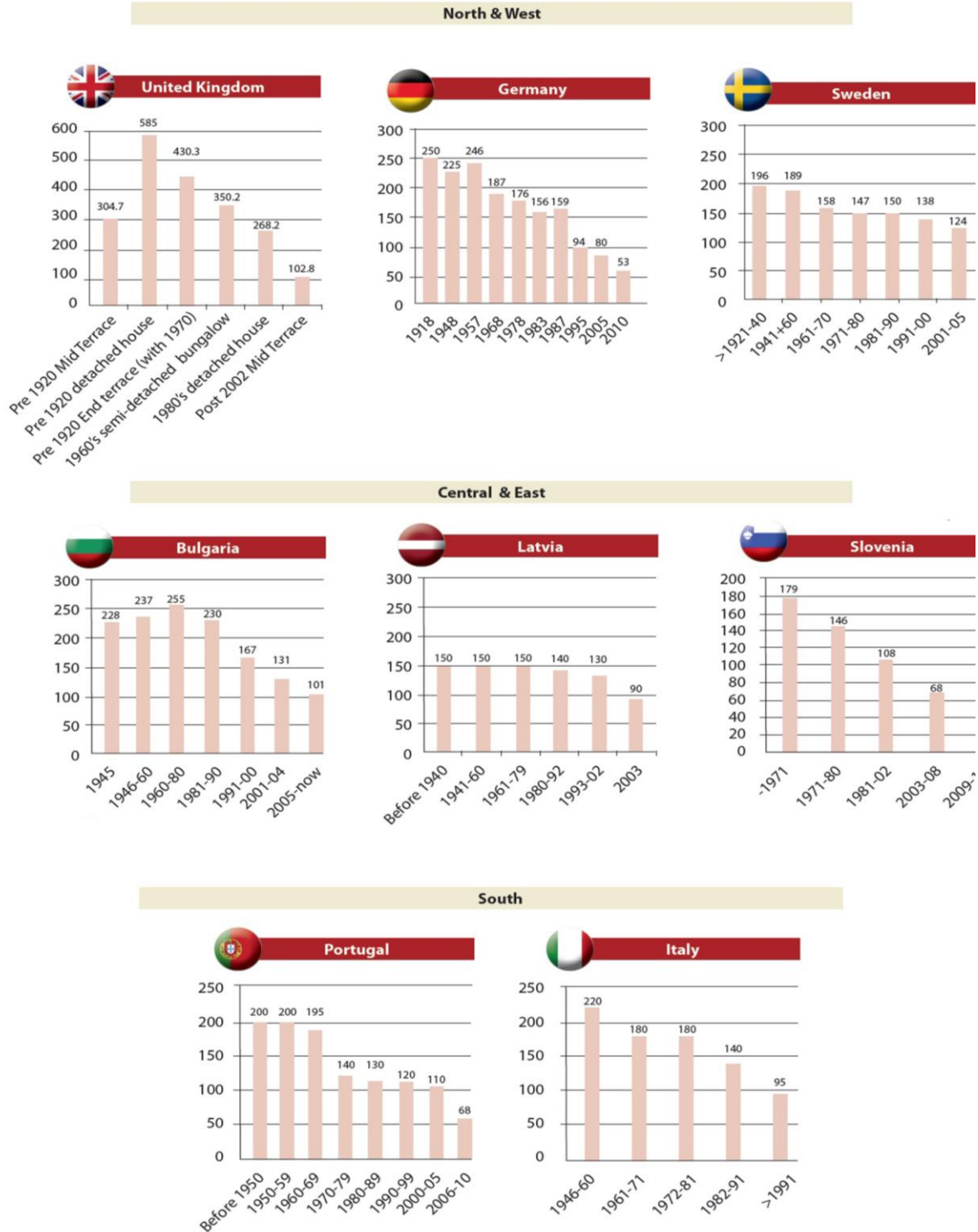
Figure 31 - Average heating consumption levels in terms of final energy use (kWh/(m 2 a)) of single family homes by construction year (BPIE, 2011)
