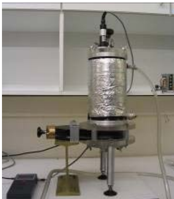
Fig. 2: Set-up of the aerosol deposition chamber
