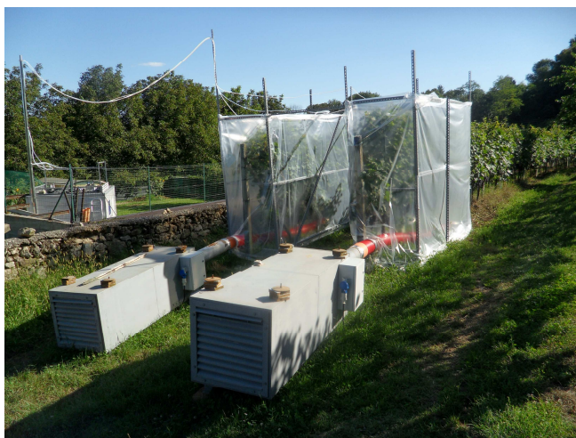
Figure 1: Two open top chambers enclosing vine grape plants on the vineyard in Angera.
