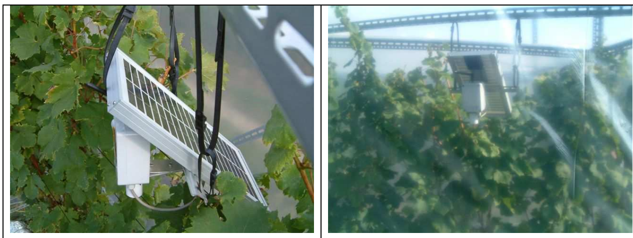
Figure 2: NanoEnvi® ozone microsensors used to monitor ozone in grape vine OTC with their solar cells used for power supply
