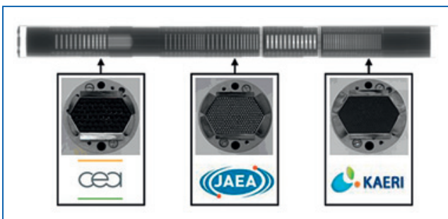
Figure 24 - Overview of the PYCASSO-II experiment by means of X-ray, and the samples provided by contributors from Europe (CEA, France), Japan (JAEA) and South Korea (KAERI)
