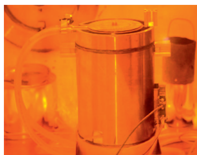
Figure 33 - Retrieval set-up for specimens irradiated in IBIS, located in the F1 cell in the Hot Cell Laboratory.
