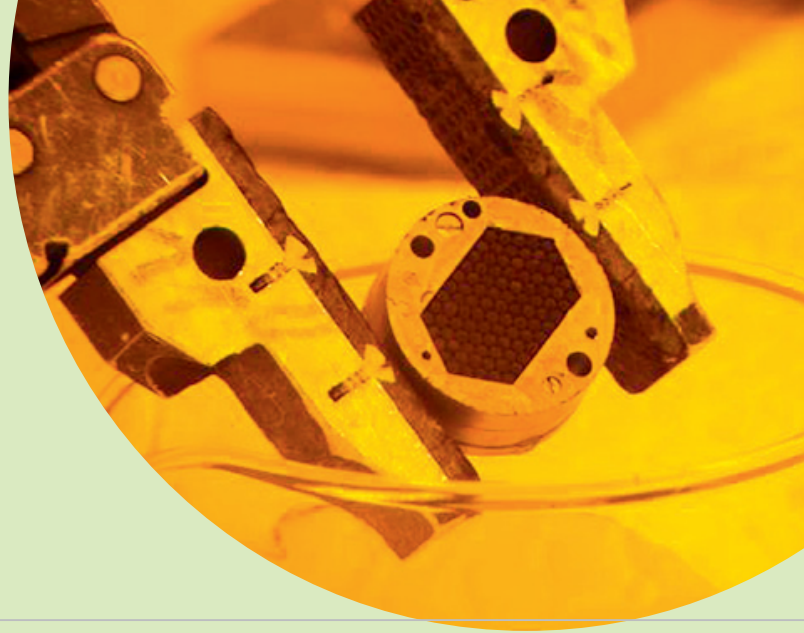
Figure 23 - PYCASSO-I dismantling, showing irradiated CEA samples in sample holder disk, in the NRG Hot Cell Laboratory
