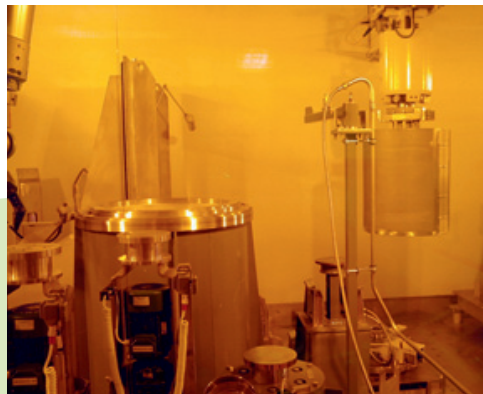
Figure 7 - The basket holding HEU elements is ready to be loaded into a canister in the hot cell at COVRA
