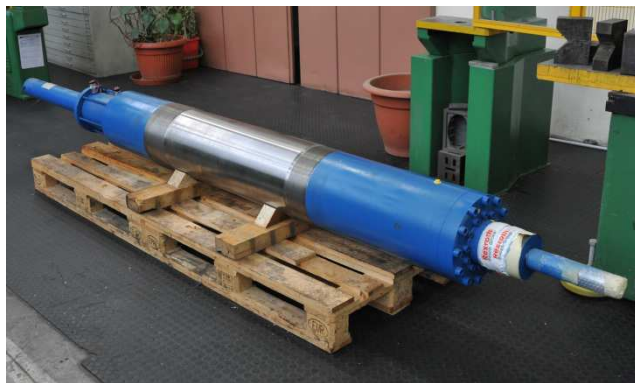
Figure 4. a) Blast actuator as manufactured by Bosh Rexroth b) nitrogen charging system
