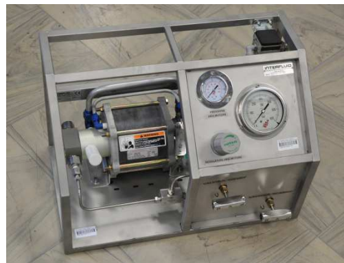
Figure 4. a) Blast actuator as manufactured by Bosh Rexroth b) nitrogen charging system
