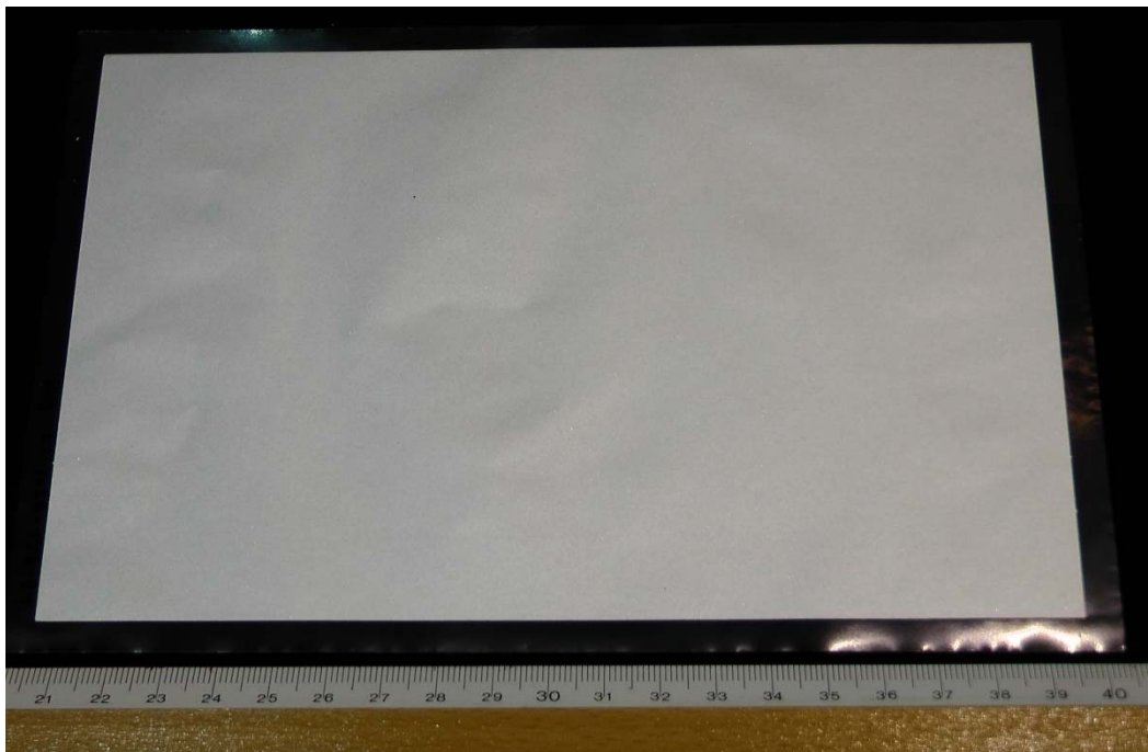
Nominal Capacitance: 85 nF Part number: 1-1004347-0 Model Description: Metallized Piezo Films [21]
