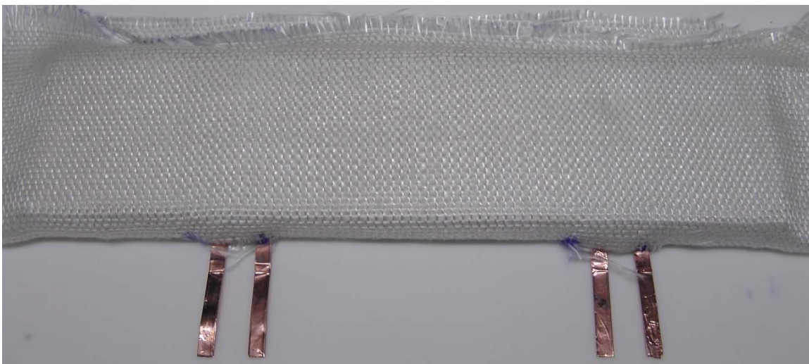
Figure 7. Preparation of sandwich specimen prior to resin infusion, with the sensor placed between the core and the composite skin.
