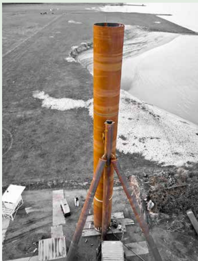
Figure 2. Fistuca: A test model with a column of water delivering reaction force for the combustion room on top of the monopile
