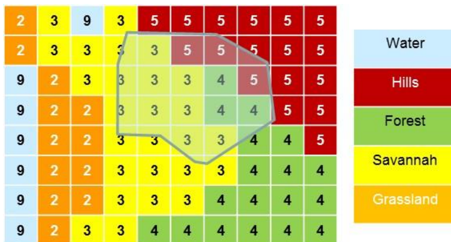
FIGURE 26. EXAMPLE OF AN ACCESSIBILITY MAP FOR A PROTECTED AREA (GREY POLYGON) WHERE LAND COVER CLASSES ARE USED TO DERIVE WEIGHTS AND GENERATE A COST-DISTANCE FUNCTION. HIGH VALUES ARE CORRESPONDING TO OBSTACLES WHILE EASIER ACCESS IS CORRESPONDING TO LOW VALUES.
