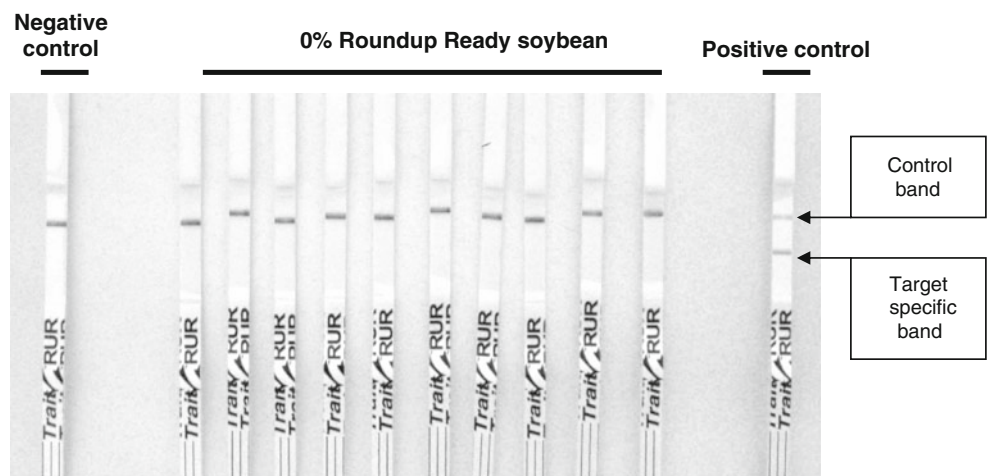
Fig. 1 Specificity of the Trait/RUR lateral flow test on flour samples of Roundup Ready soybean (Certified Reference Material, 0 % series 410R); negative control : water; positive control : 5 % RUR soybean
