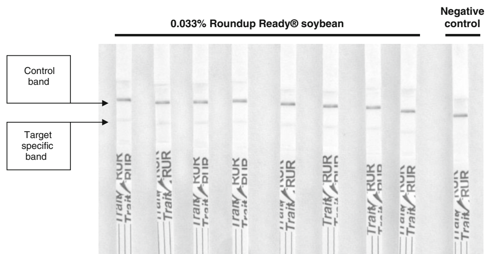
Fig. 2 Assessment of the sensitivity of the Trait✓ RUR lateral flow test on replicated samples prepared at 0.033 % (w/w) GM Roundup Ready soybean; the specific band is indicated by the arrow; negative control : water. For details on lateral flow strips detection procedure see “Materials and Methods”
