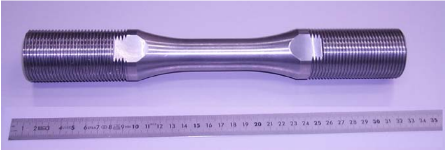
Fig. 10. Steel dumb-bell shaped specimen of 30 mm diameter.
