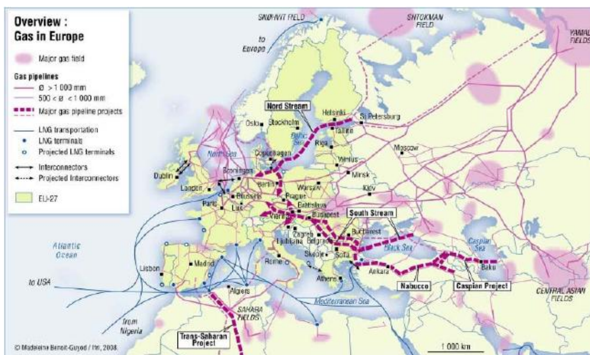
Fig. 4.7 Overview of the gas networks in Europe (Nies, 2008)
