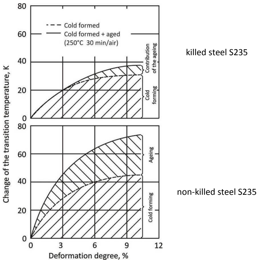
Figure 6-4: Ageing effects of rolled steels [9]
