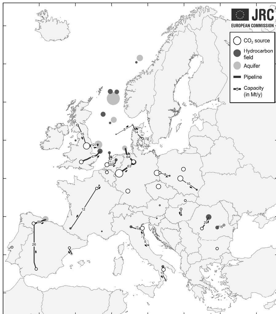
Figure 5.2: CO 2 pipeline network in 2050, assuming individual optimisation per country, without international cooperation. Total amount of CO 2 captured and stored: 565 Mt/y.
