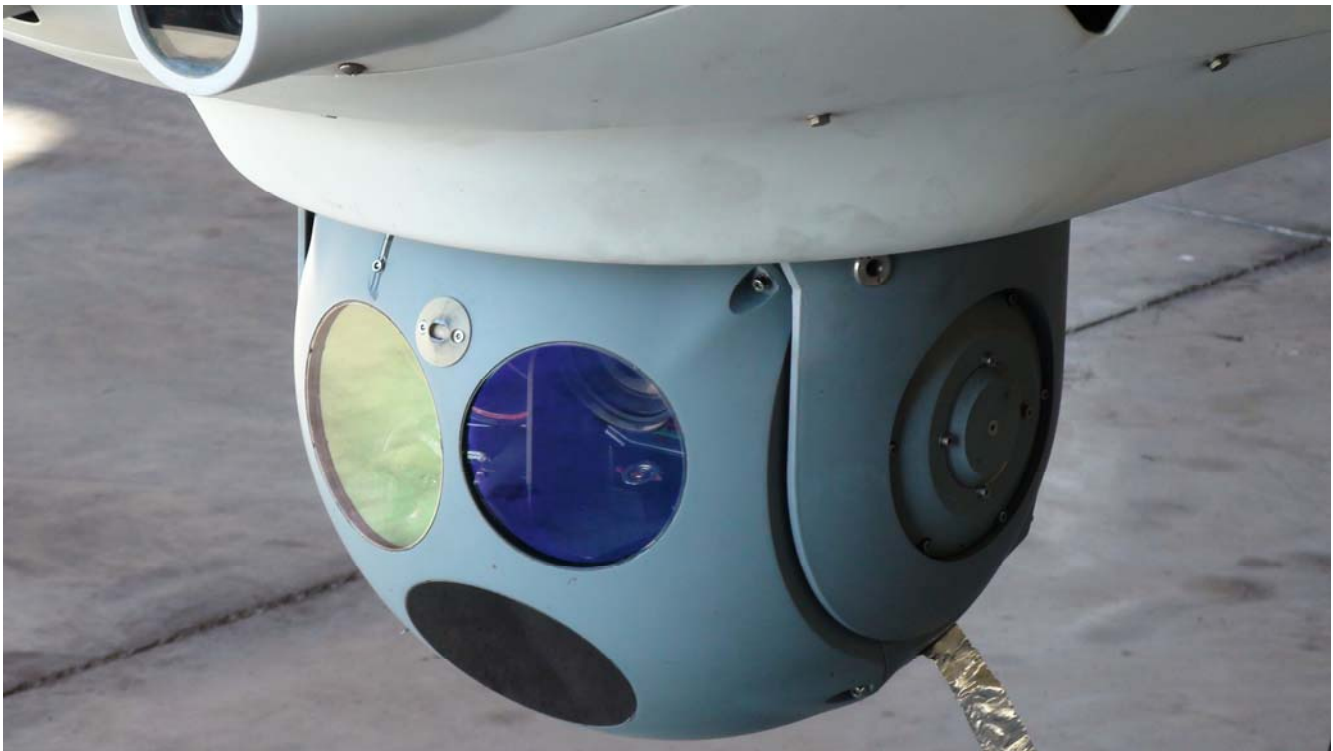
Figure 10 – The payload of the Sky-Y was the Selex Galileo EOST Galileo 45, which comprises an Electro-Optical InfraRed (EO/IR) stabilized Turret, stabilization (4 axis), 20 \mu rad, an IR Camera (2 FOV) 3-5 \mu m, Colour TV Camera (Visible), Spotter (Visible) and a Laser Designator (option). The total weight is 35kg.
