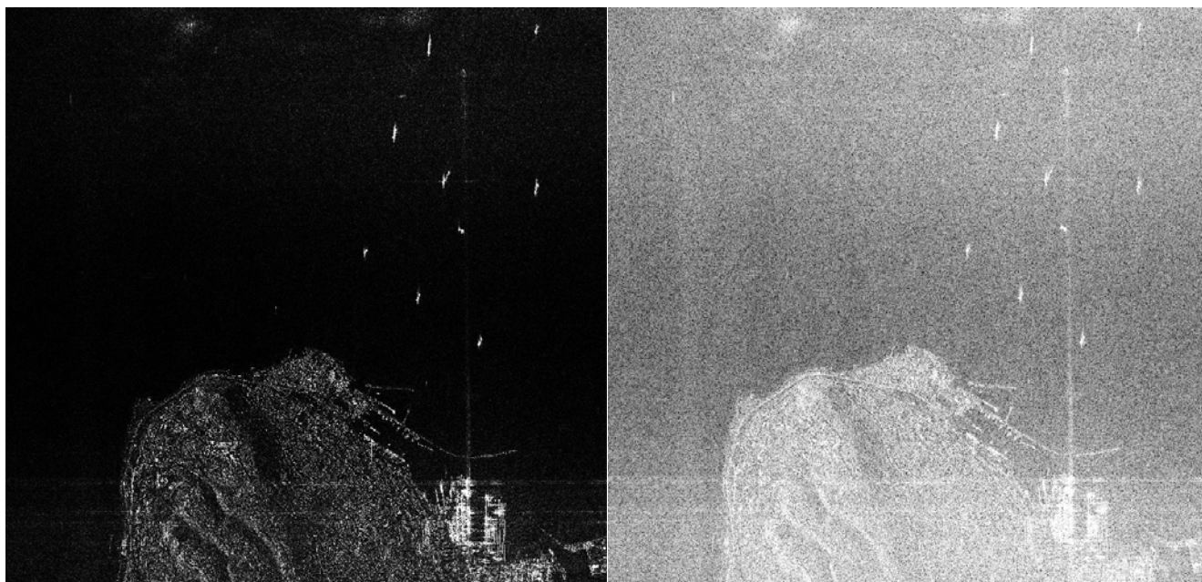
Figure 21 – Radarsat-2, Spotlgiht image (08Dec.2010) - On the left, the Sigma Naught ( \sigma^\circ ) (intensity) and on the right, the Sigma Naught ( \sigma^\circ ) (dB).
