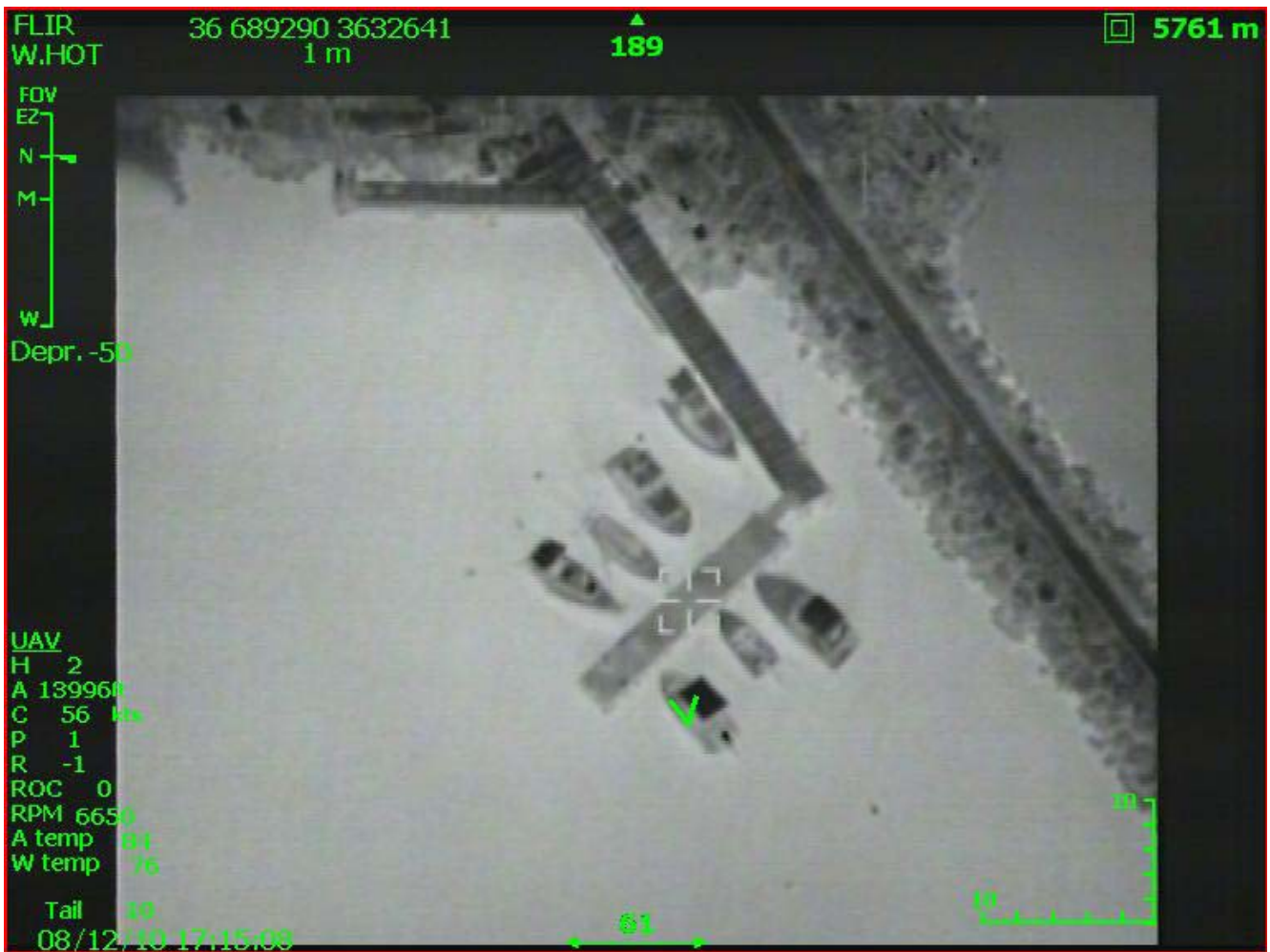
Figure 19 – UAV IR image of a small pier in the port of Haifa, Israel where 7 small boats can be seen with enough detail to allow classification. This image was acquired from an altitude of about 5,500 meters in the dark.
