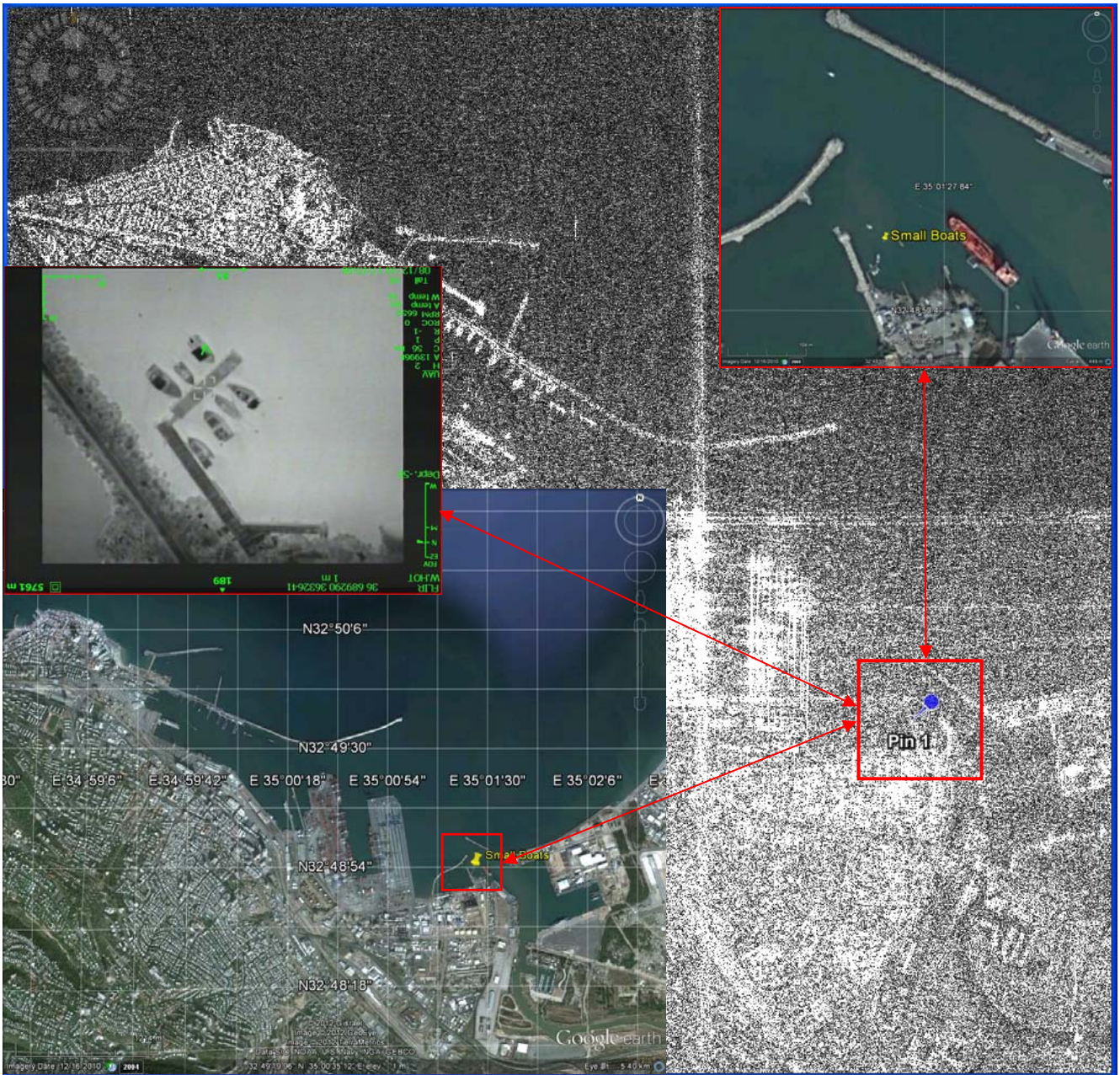
Figure 18 – Photo taken in Haifa Israel a couple of hours before the SAR satellites overpass. This photo shows the large ships moored in the area. Most of these large ships were detected in the Radarsat-2 image. As expected their positions and orientations were slightly different at the time of the satellite overpass.
