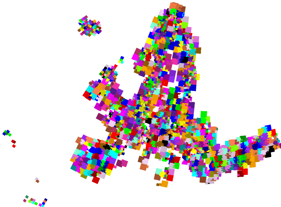
Figure 2: Labelled decision regions for the first coverage based on CROIs (1944 images used in mosaic out of 2004).
