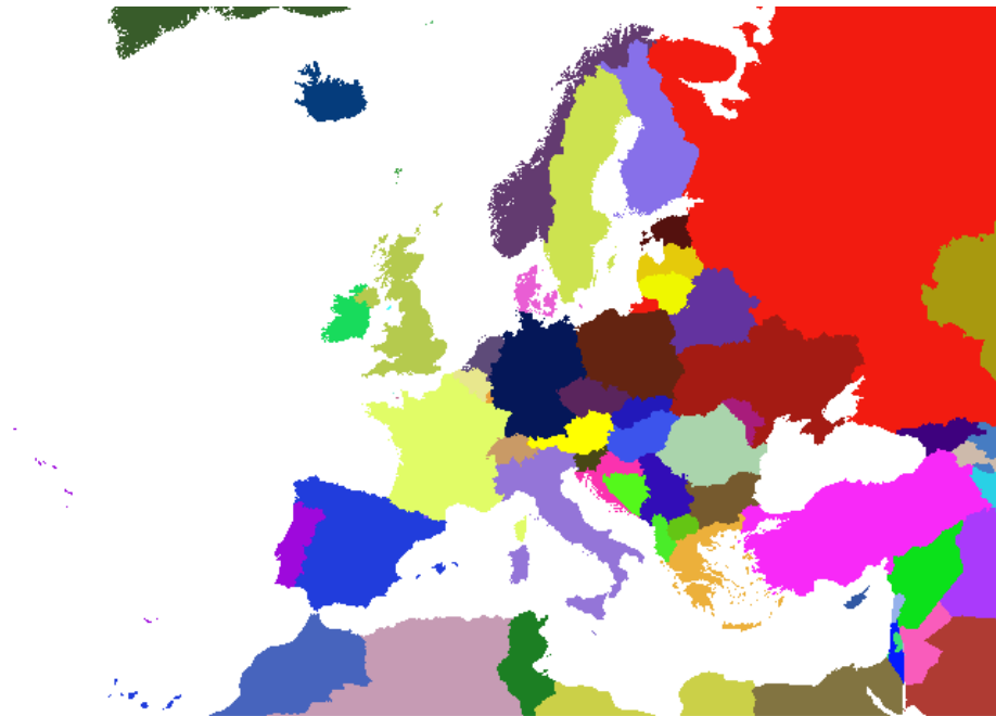
Figure 1: Gisco version 9 NUTS0 vector file rasterised at 250m using ETRS-89 LAEA projection and the European grid. Serbia (code RS) and Montenegro (code ME) still appear within the same unit (dark blue region in the Balkan Peninsula).
