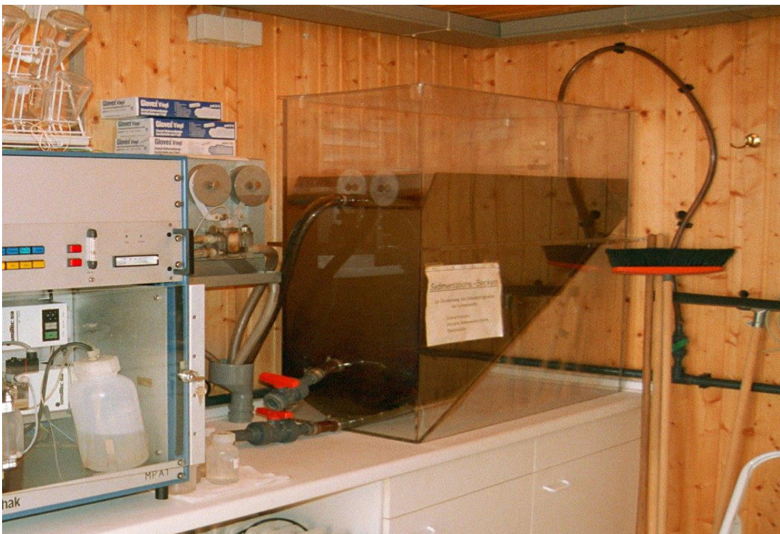
Sedimentation chamber in a monitoring station for collecting freshly deposited sediment "FDS" (composite sample, FGG Elbe 2008)
