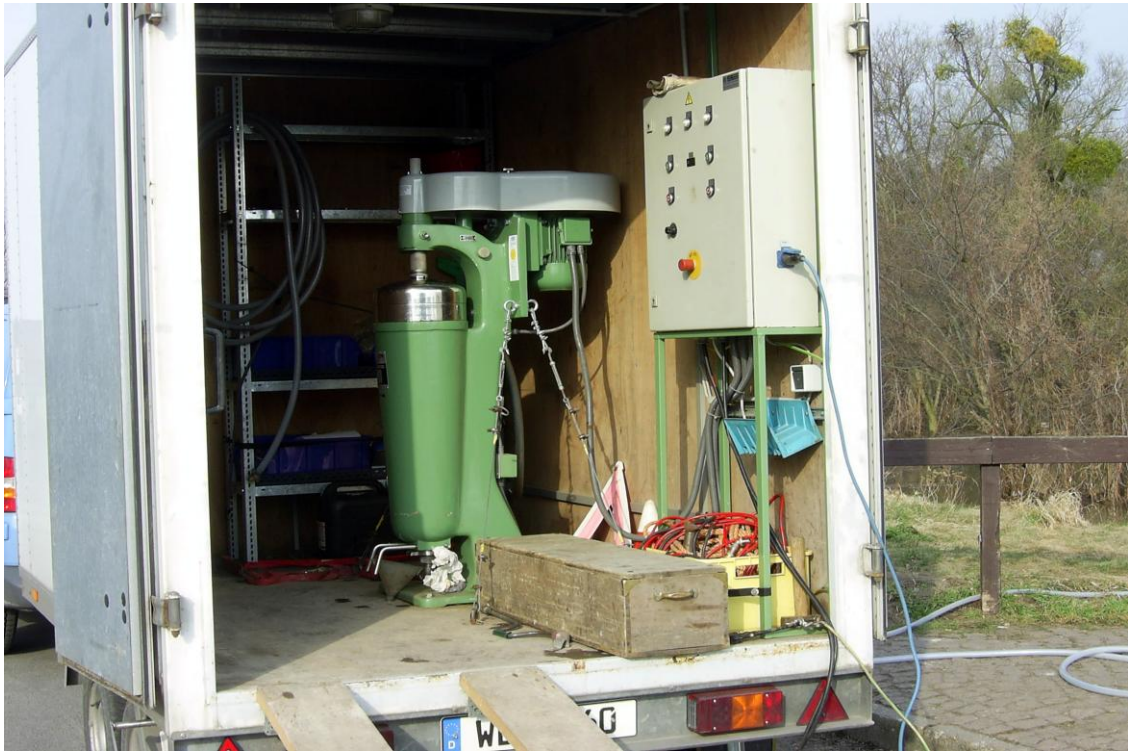
Continuous centrifuge for sampling SPM (LHW, Labor Wittenberg 2010)
