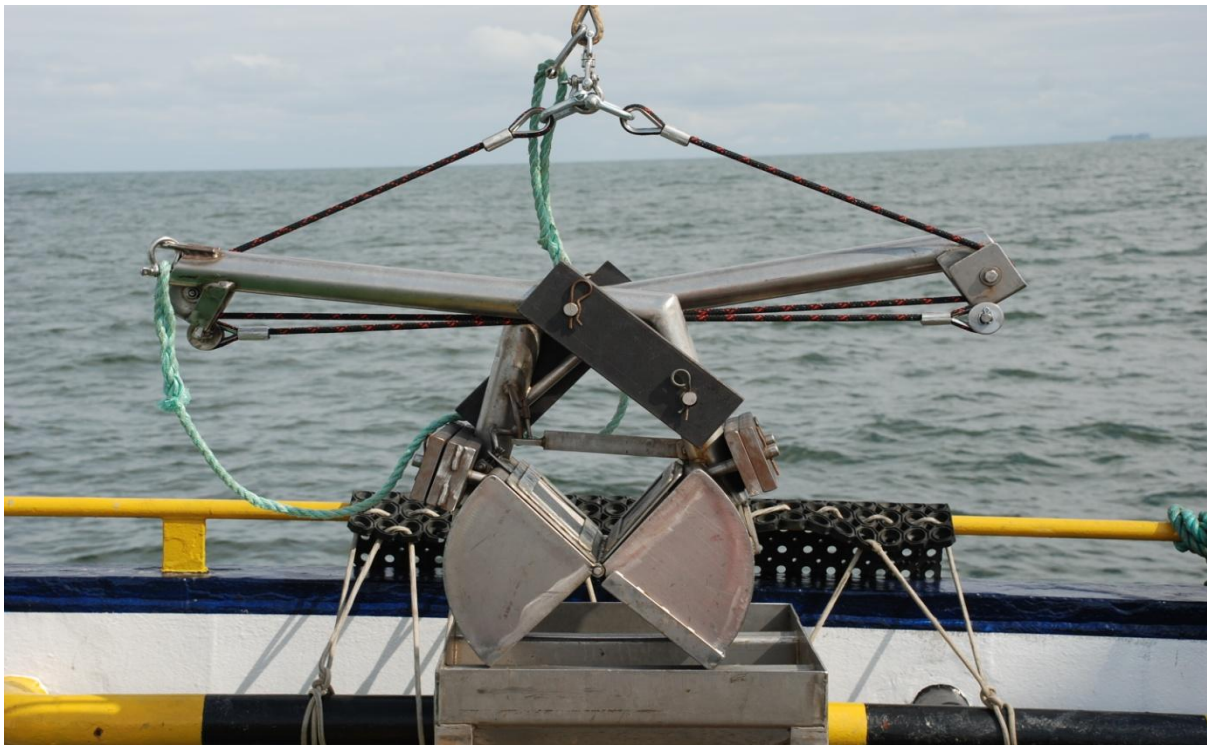
Van-Veen grab for sampling surface sediment samples (Hamburg Port Authority 2011)
