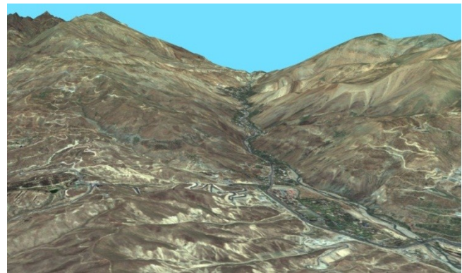
Figure 21: 3D visualization of digital surface model of Teheran from WV2 stereo pairs with texture from MS channels.
