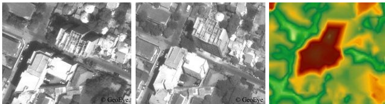
Figure 16. Example of corridor occlusion due to tall buildings; (a) and (b): stereo images; (c) resulting DSM (Dakar).
