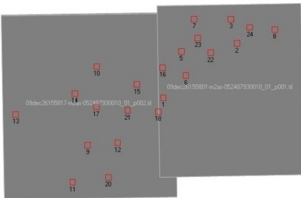
Figure 27. Dakar project. Location of GeoEye stereo-pairs (in grey with white border) and manually measured tie points (red squares).
