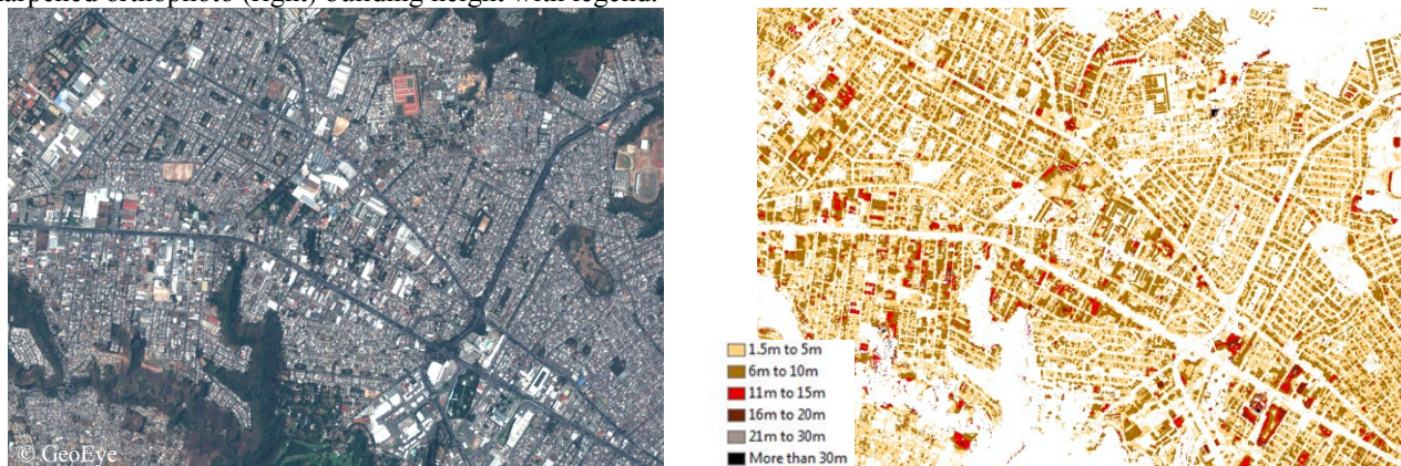
Figure 25: Automatic building height extraction in Guatemala City from stereo images. (left) pan-sharpened orthophoto (right) building height with legend.
