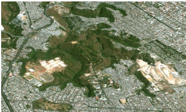
Figure 20: 3D visualization of digital surface model of Guatemala City from GE1 stereo pairs with texture from MS channels.
