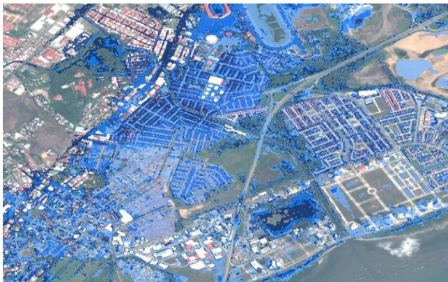
Figure 18. Flood simulation in North-East of Panama City using WV2 DSM.
