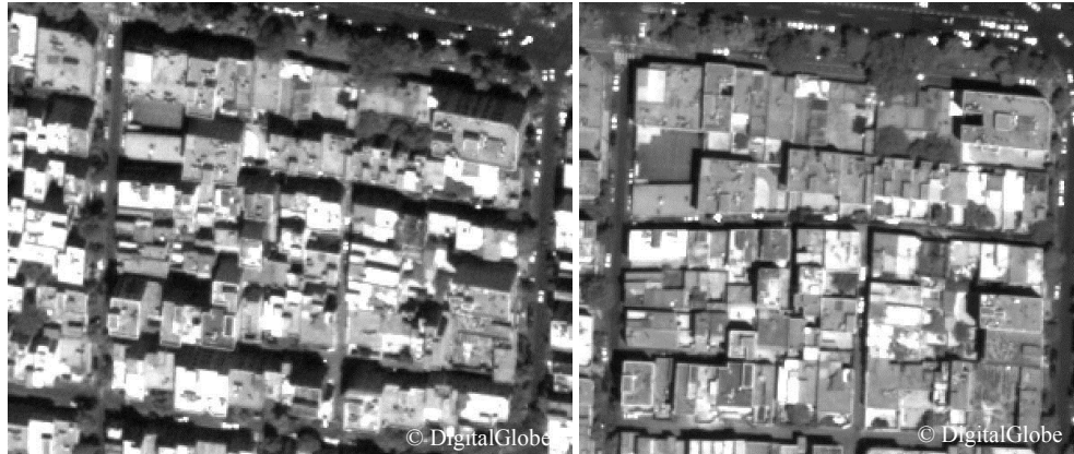
Figure 1. Stereo image acquisition in Teheran project. Left: forward viewing direction 27^\circ , right: nadir viewing direction. The time difference between the two acquisitions is about one minute.
