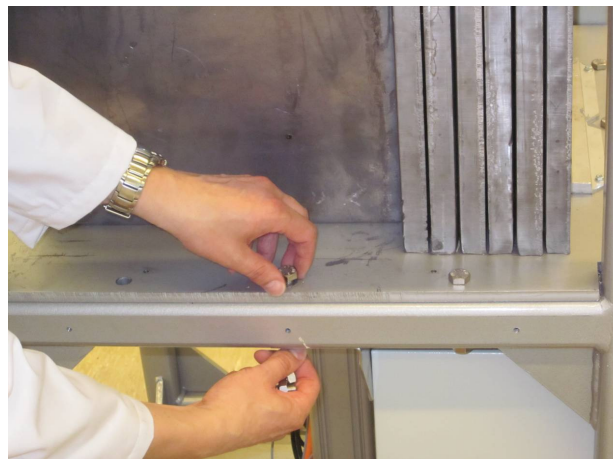
Figure 13: Nuts and bolts to fix the base plate.
