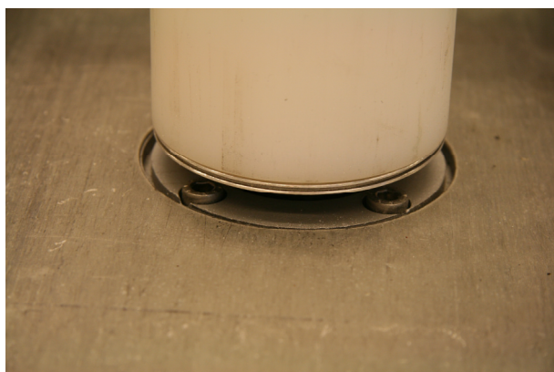
Figure 53: Source holder in homing position (NIR – neutron).
