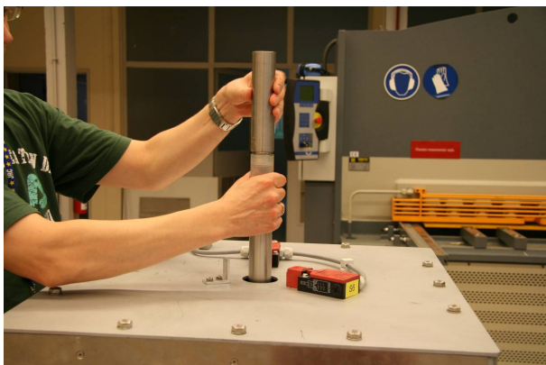
Figure 30: Unscrew top of source holder
