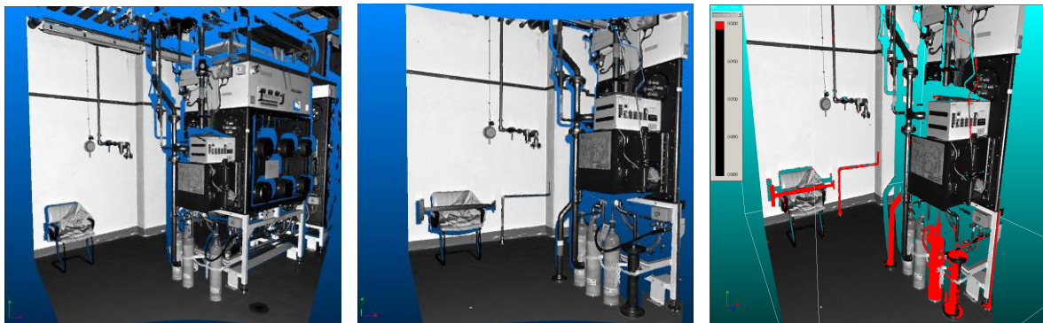
Figure 2: Reference model (L), verification scan (M), automatically detected differences in red (R)
