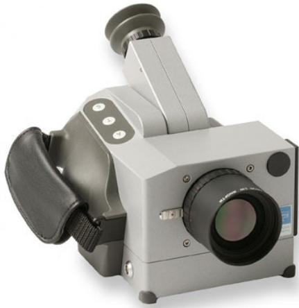
Figure 5: Off-the-shelf infra red camera as used by IAEA for IR imaging (temperature resolution 0.1 K at 30 C, measurement accuracy \pm 2\% over –measurement range -40 C to 1200 C)
