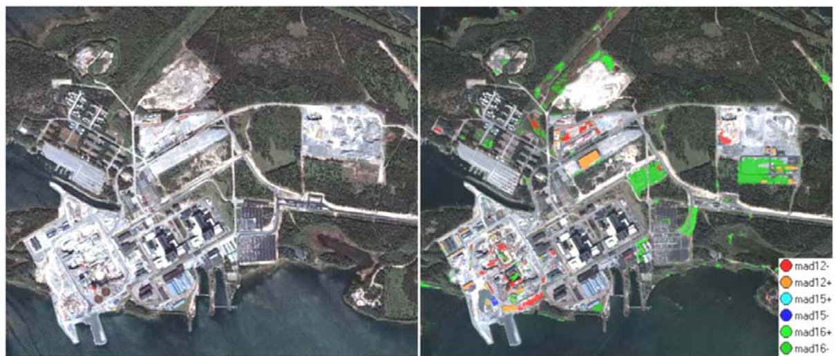
Figure 5: Results of the object-based change detection for Olkiluoto between June 2005 (left) and July 2006 (right) based on 16 objects, given by the MAD layers 12, 13 and 16 (right)
