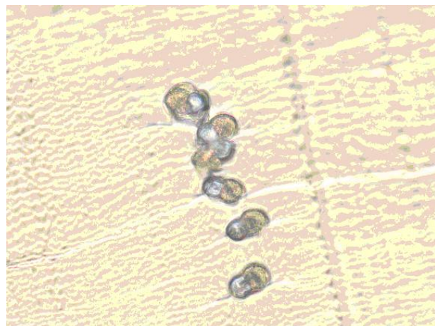
Fig. 1: Pure elastomultiester (sample 021 ) after dyeing at 100 °C. 400X. a) longitudinal analysis; b) cross-section analysis.
