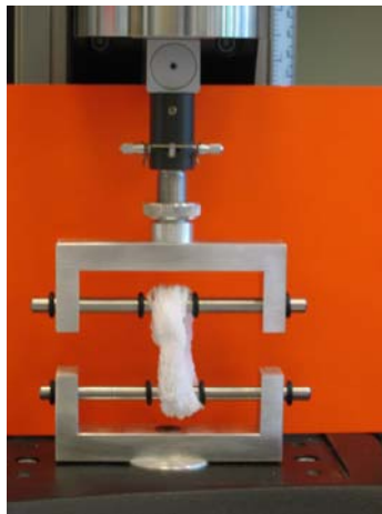
Fig. 11: Clamping assembly used for the skein method.
