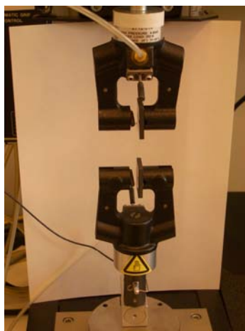
Fig. 8: Clamping assembly used for the BISFA method.
