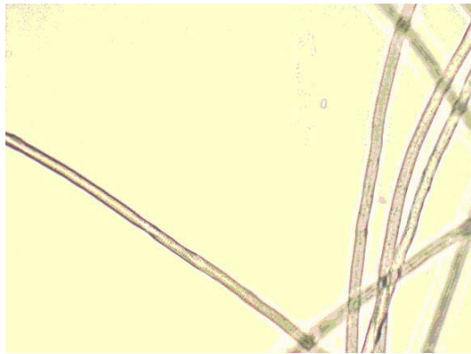
Fig. 25: Pure polyester extracted by sample 048 . 200X and 400X.
