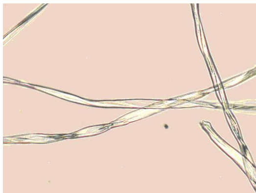
Fig. 23: Pure cotton extracted by sample 054 . 200X and 400X.
