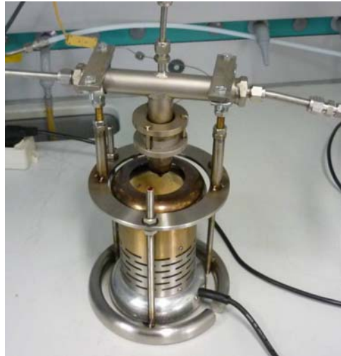
Figure 10: JRC's homemade oil particle generator
