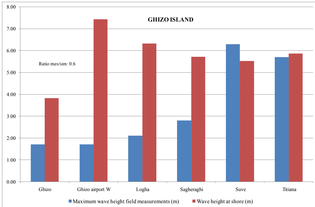
Figure 37. Ghizo Isl. Maximum wave height simulated with HYFLUX2 (red) compared with field measurements. (blue)
