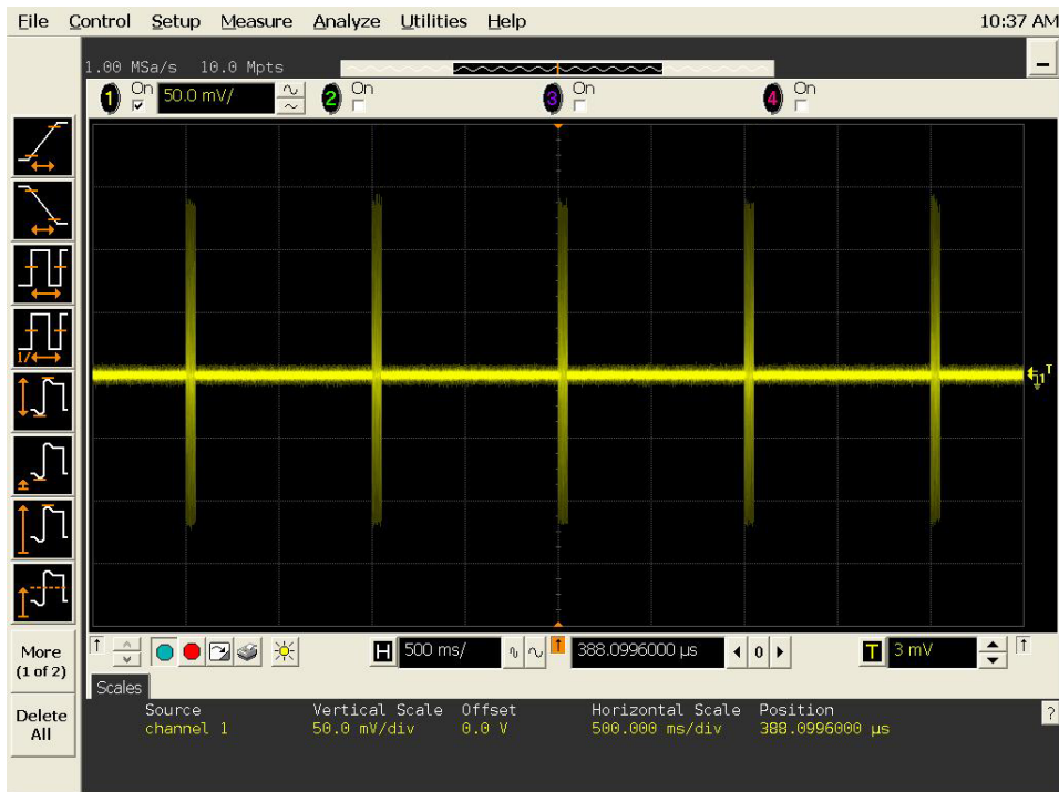
Figure 29: MB-OFDM UWB LDC signal (Duty cycle: 5%, T_{on} = 50 ms, T_{off} = 950 ms)
