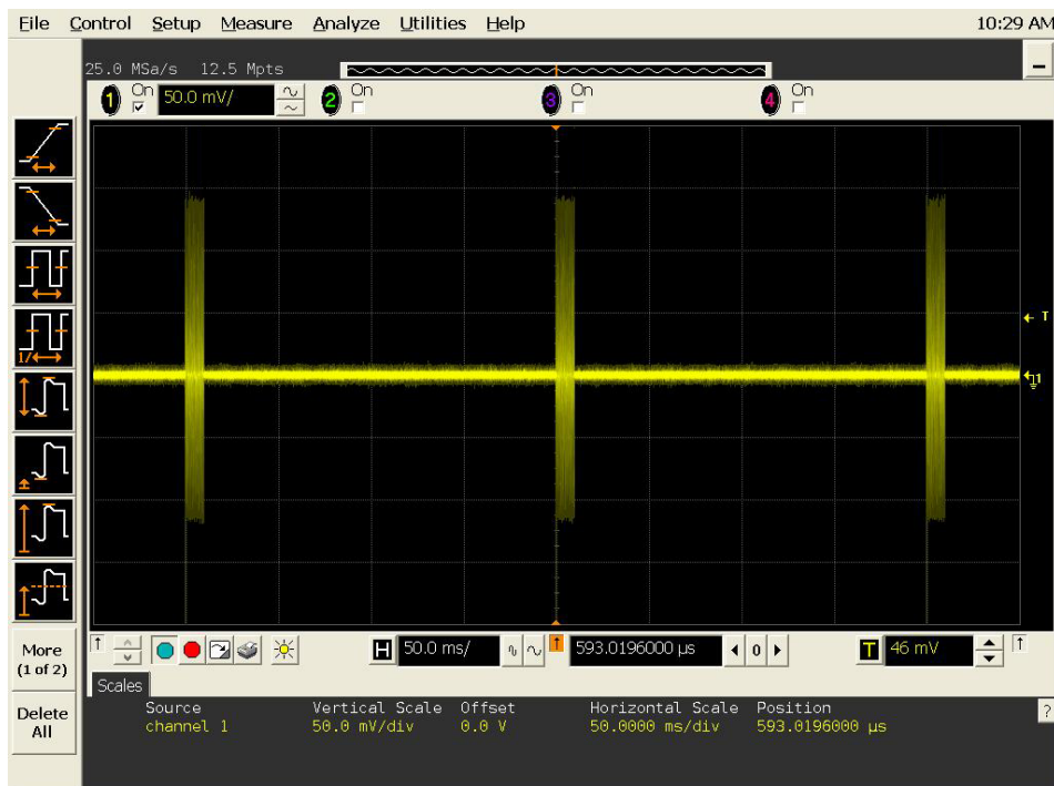
Figure 27: MB-OFDM UWB LDC signal (Duty cycle: 5%, T_{on} = 10 ms, T_{off} = 190 ms)
