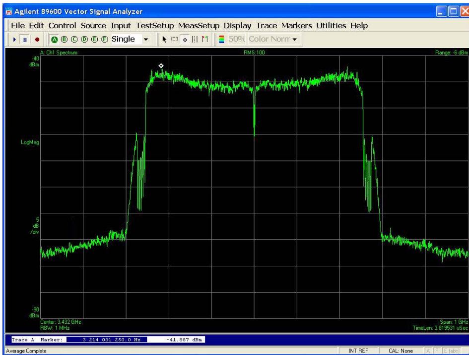
Figure 23: MB-OFDM UWB test signal spectrum
