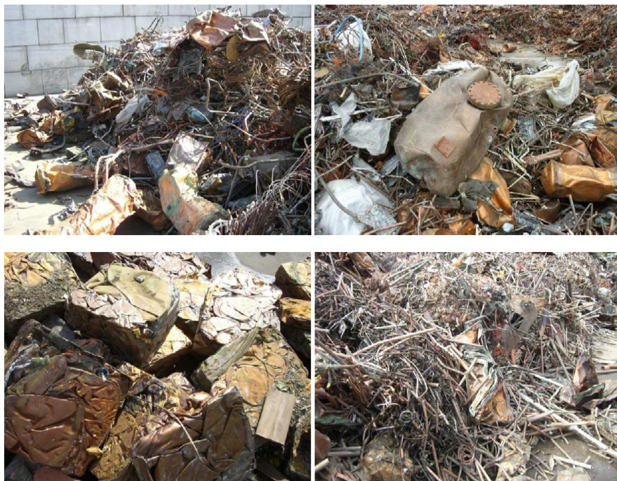
Figure 8: Examples of No 2 copper scrap with foreign material content between 5 to 10 %. Source: Aurubis, 2010.
