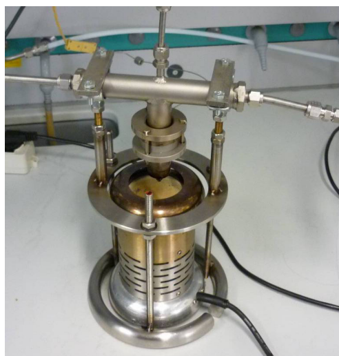
Figure 9: JRC's homemade oil particle generator
