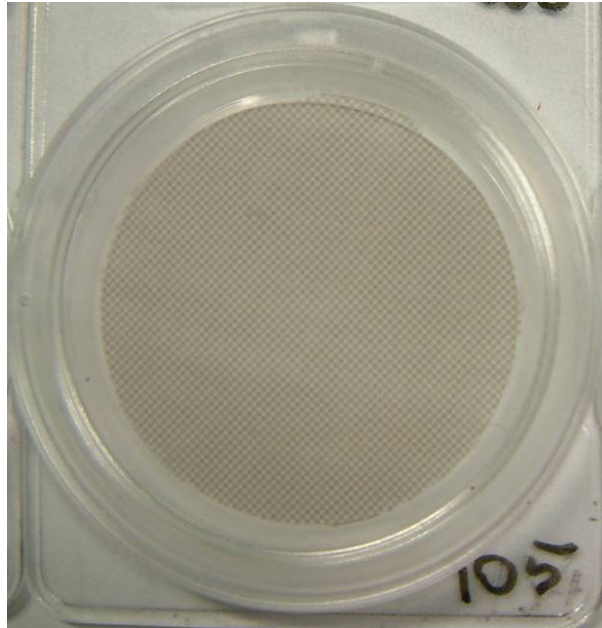
Figure 52: Loaded Teflo filter collected from the m-PSS from an ESC 12 test at 10% valve opening.
