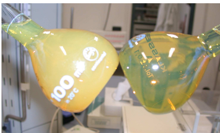
Figure 20: Top (right) and bottom (left) diluted test portions.
