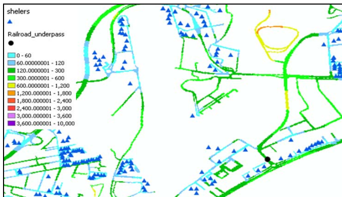
Figure 11: Map of distance classes from closest shelter (Mandelieu test site); yellow to red coloured areas are the most distant road segments in this example
