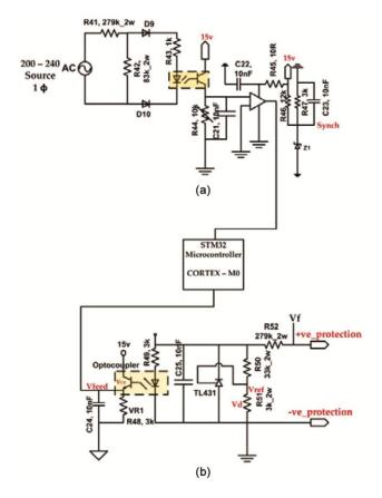
Fig. 3 — (a) Zero voltage detector circuit; (b) Line regulation circuit)
