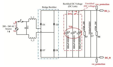
Fig. 1 — Schematic diagram of diode bridge rectifier for digital control plasma switching power supply
