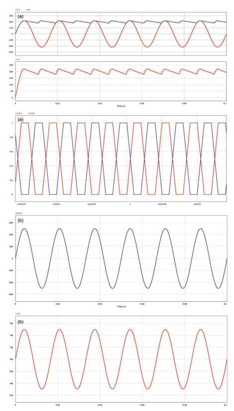
Fig. 4 — Simulation results of power supply circuit: (a) input power supply  $(V_{AC})$ , DC voltage  $(V_{DC})$  and rectifier voltage  $(V_{PC})$ ; (b) Transformer primary voltage  $(V_{PC})$ , and output voltage  $(V_{DC})$  and output voltage  $(V_{DC})$  and rectifier voltage  $(V_{DC})$ .
