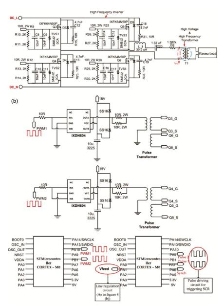
Fig. 2 — Schematic diagram of PWM inverter for digital control DBD AC power supply (a) power source; (b) Driver circuit with STM microcontroller
