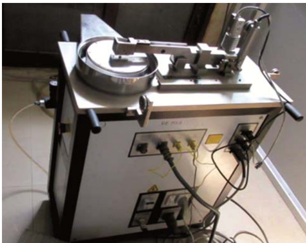
Fig. 5 (a) — Pin-on-disc test set-up.
