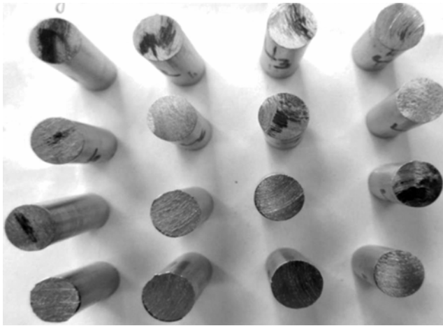
Fig. 6 — Worn surface of uncoated IN800 substrate.
