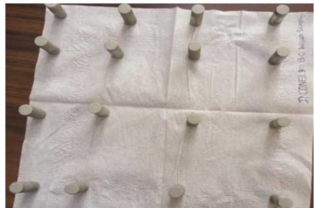
Fig. 2 — As-air plasma sprayed bond coated samples before sol-gel deposition.
