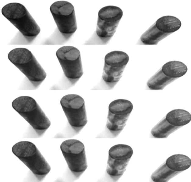
Fig. 7 — Worn surface of coated IN800 SGTBC.
