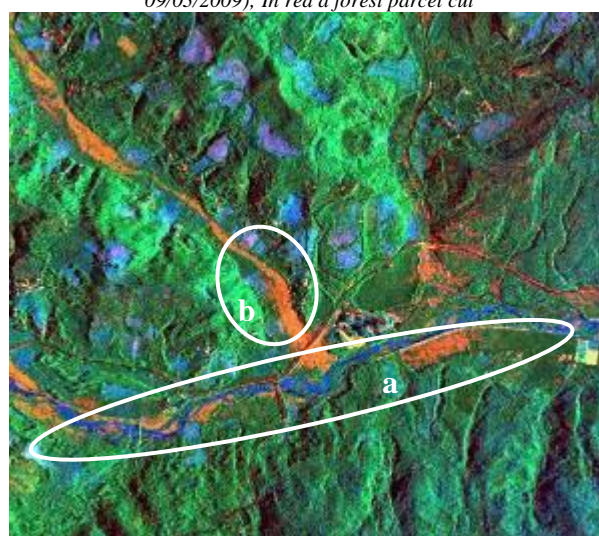
Figure 14 ILU done over the Pollino area ((COSMO-SkyMed Spotlight-2 interferometric couple: 08/12/2008-09/03/2009); Changes on the river path are in blue due to the high differences on the backscattering values over the flooded or dried areas within the two acquisition (a). The dried river-bed appears in red because, being characterized by rocks, has a high level of coherence (b).
