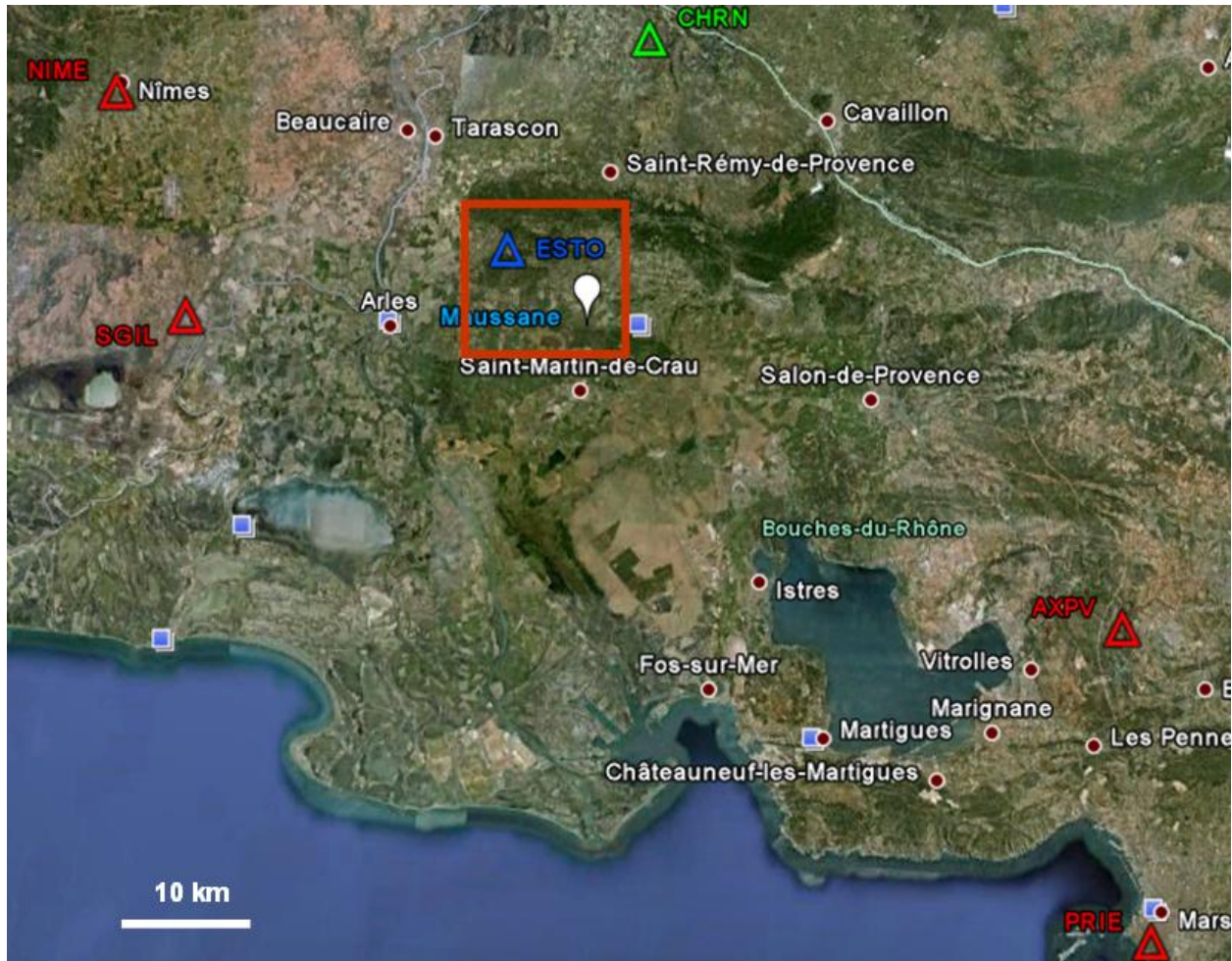
Figure 2. Available base stations near from our test site area: in red RGP (SGIL, NIME, AXPV, PRIE), in green RENAG (CHRN), in blue our BS settled in Chateau d’Estoublon domain. The Marseille BS is included in EUREF network.
