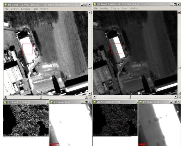
Figure 7. Effects of linear stretching applied to forward scene for 11-to-8-bit reduction. Left: after linear stretching (8 bit), right: before linear stretching (11 bit).
