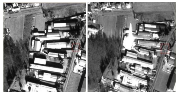
Figure 8. Sensor saturation problems. Left: forward scene, right: reverse scene.
