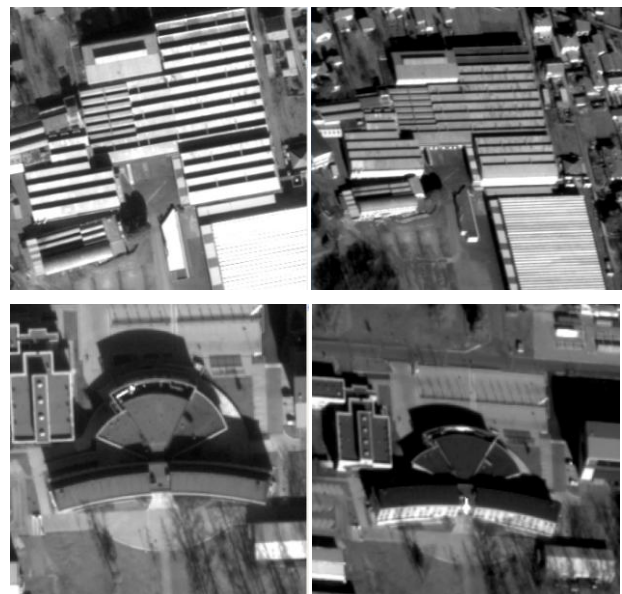
Figure 4. Scale and radiometric changes between forward (left) and reverse (right) views.
