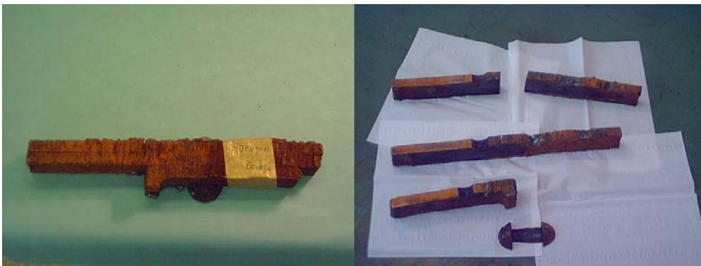
Figure 11. The "Yokogawa bridge" sample as arrived and disassembled,
