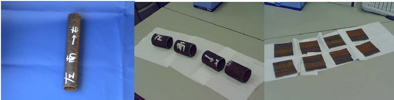
Figure 10. The "Kyu-Fuzoku elementary school" sample as it arrived, cut in pieces and these pieces cut longitudinally and flattened.
