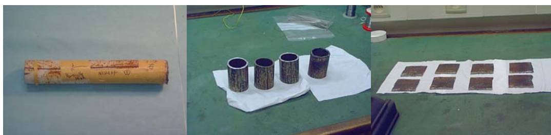
Figure 16. The "Nisseki 5" sample as it arrived, cut in pieces and these pieces cut longitudinally and flattened.
