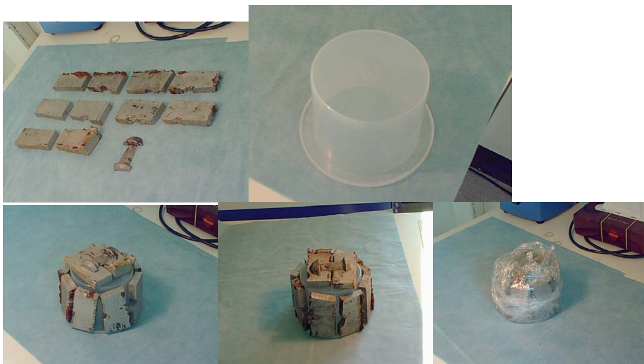
Figure 12. The "Yokogawa bridge" with its pieces cut and cleaned, the inner part of a Marinelli beaker and the sample arranged around it and fixed with plastic foil for measurement.
