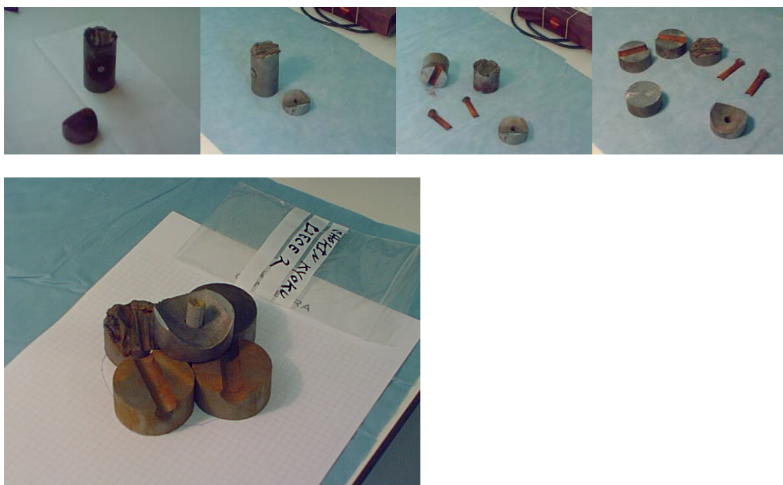
Figure 17. The "Postal Saving Building" sample separated in its components, these when cut in pieces and cleaned and the connecting pin cut longitudinally
