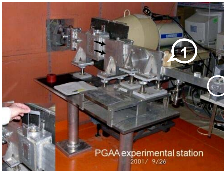
Figure 1. The PGAA and NIPS beam tubes. The two neutron beams are indicated by the two black arrows. They are inside the aluminium tube which is lined with Li-6 polymer neutron-absorbent sheets to decrease the flux of escaping scattered neutrons. The upper (PGAA) beam is stopped by Li-6 polymer sheets at the end of the upper section (indicated by 1). The lower beam continues to the NIPS station indicated by a circle. The sample holder and the placing of a sample in the target chamber are shown in the lower-left insert.
