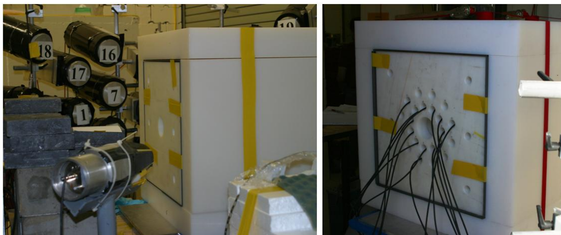
Figure 5. Installation of the setup on the beam line. The left part shows the front side of the counter with the beam arriving from the left. The right part shows the rear side with the two concentric rings of tubes around the beam axis. The external shielding can be seen with the boron carbide (black plates) between the two blocks of polyethylene. The shielding of these front and rear faces was not yet installed on these pictures.
