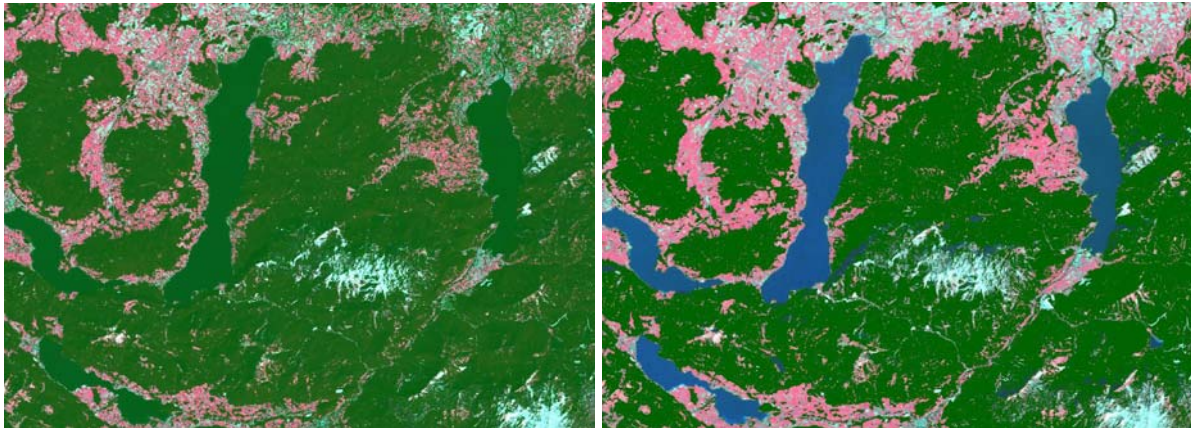
Figure 5-19: Example of the effect of using the spectral distance-parameter: kNN forest map around Attersee and Traunsee (A) using German inventory data without (left) and with (right) using the parameter of spectral distance
