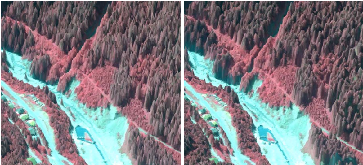
Figure 5-12: Left: 3D-view of an Orthophoto where ALS data was used as height information. Right: 3D-view of an Orthophoto where the DEM derived from the Ultracam data was used as height information.
