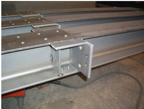
S235JR Construction class II Detail class B
