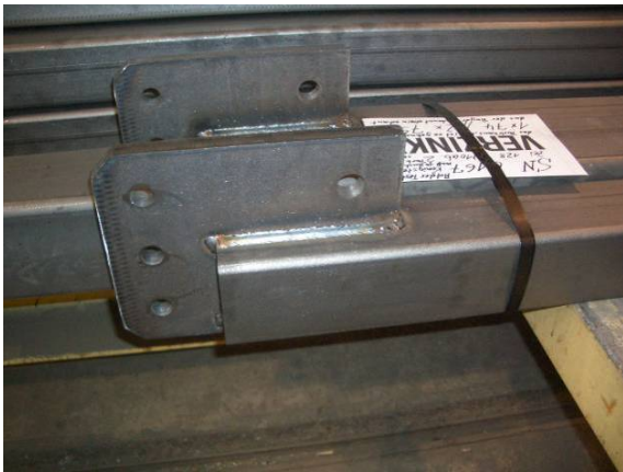
S355J0 Construction class I Detail class C
