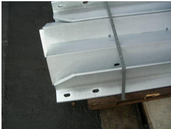
S235JR Construction class I Detail class B
