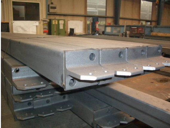
S355J0 Construction class I Detail class A
